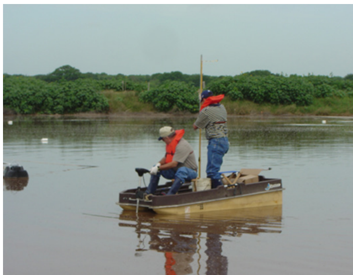
Figure 12. Depth profile sampling work at a dairy lagoon with two people in a flat-bottomed boat. Photo from Mukthar et al. (2009), used with permission.
