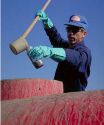
Figure 8. An example of using a cup-pole sampler to sample manure from a tanker. Photo from University of Minnesota Extension, used with permission.
