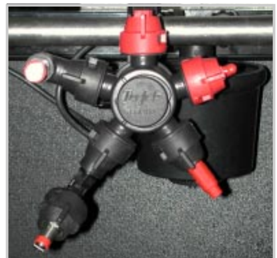
Figure 3. Illustration of a nozzle body that can accommodate multiple sprayer nozzles
