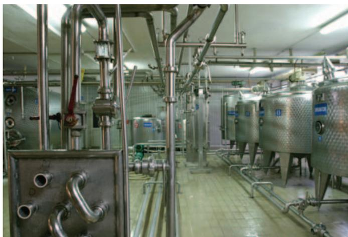
Vat pasteurization carries with it the additional challenge of rapidly cooling the milk again following pasteurization.
