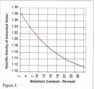
however, it does not retain its original volume, but is slightly compressed. As shown in Figure 2 (MacLean, 1952), the specific gravity of the water imbibed into wood at the f.s.p. is 1.115 (Skaar, 1972). The specific vol-
