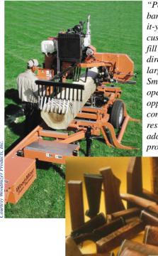
"Personal scale" band mills allow doit-yourselfers to custom cut wood to fill niche markets not directly serviced by larger sawmills. Small band mill operators have the opportunity to convert logging residue into valueadded wood products.
