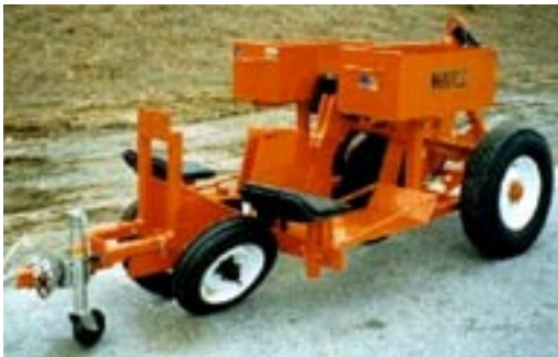
Figure 5. Tow-type transportable transplanter
