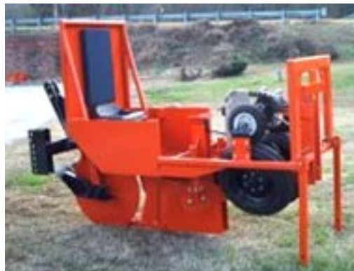
Figure 7. Semi-automatic hardwood transplanter
