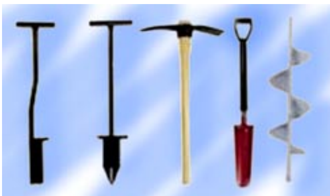
Figure 4. Tools used for hand planting bare-root hardwood seedlings. (Left to right, dibble bar, planting bar, mattock, sharpshooter shovel, and auger)
