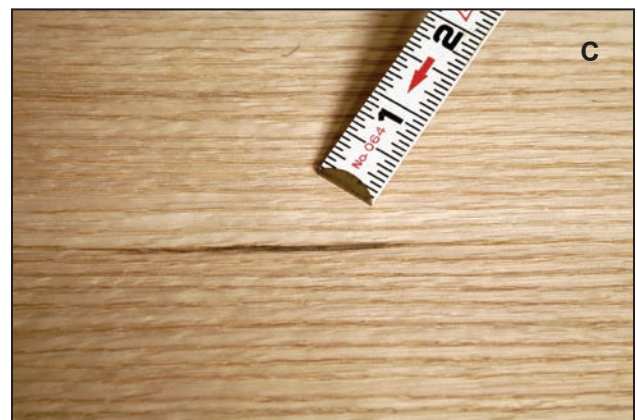
Figures 17A, B, C. Two examples of mineral stain in the end of two different red oak logs and in the veneer.
