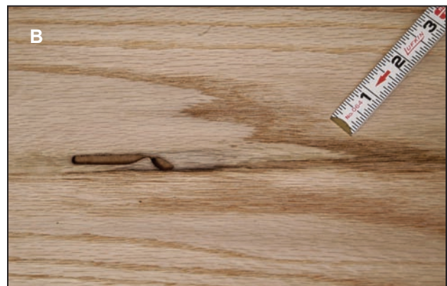
Figures 15A, B. Bore damage in the butt of white oak. This log also exhibits slow and fast growth rate, ring shake, and very poor color. Bore damage in red oak veneer is also shown (B).
