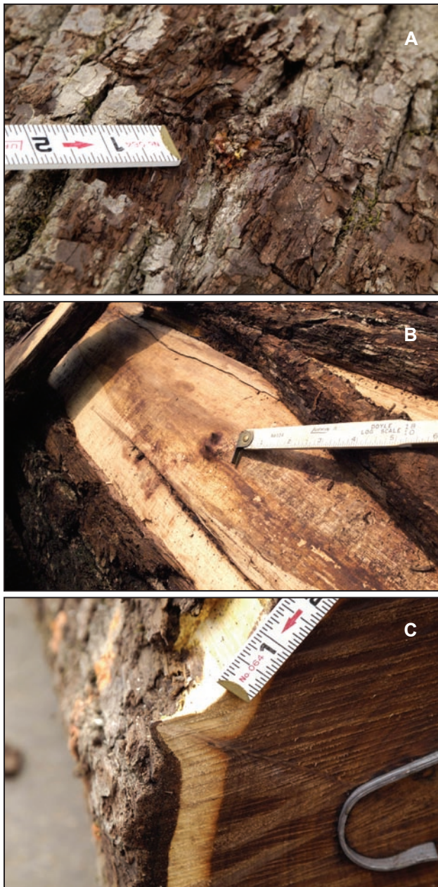
Figures 8A, B, C, D, E. Pin knots in black walnut are another troublesome defect. A shows a pin knot or cluster of knots in the bark. B shows the same type of defect with the bark removed. C shows a pin knot on the end of a log. D shows a pin knot on a flat slice of veneer, and E shows the flash or grain deviation for a pin knot on a quartered surface.
