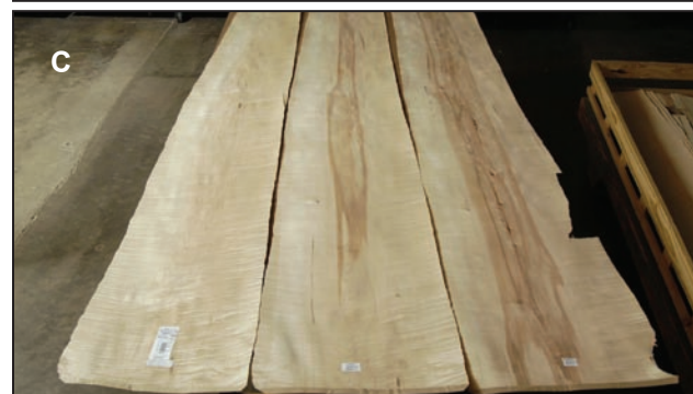
Figures 19A, B, C. The end of a hard maple log shows a very small heartwood which is good. The log end also shows two or more “black lines” or mineral streaks in the lower left quadrant. These black lines result in streaks in the veneer (B). The veneer from a different log shows the objectionable brown heartwood in contrast to the white sapwood (C).
