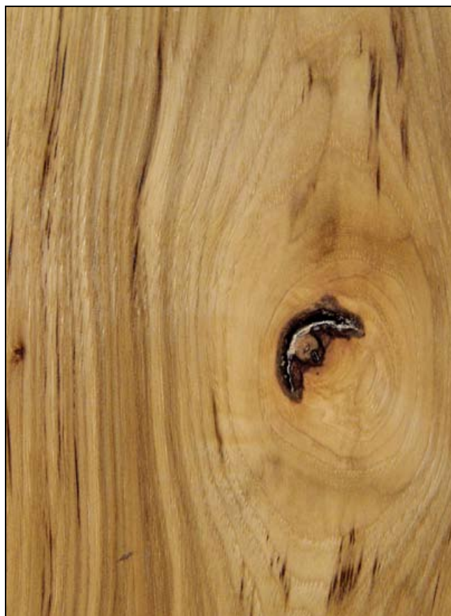
Streaking and existing bark around a knot are characteristic of hickory.
