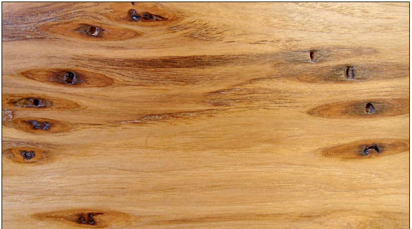
Bird peck and associated discoloration in hickory. Whitish inclusions as seen in the pores here are not uncommon.
