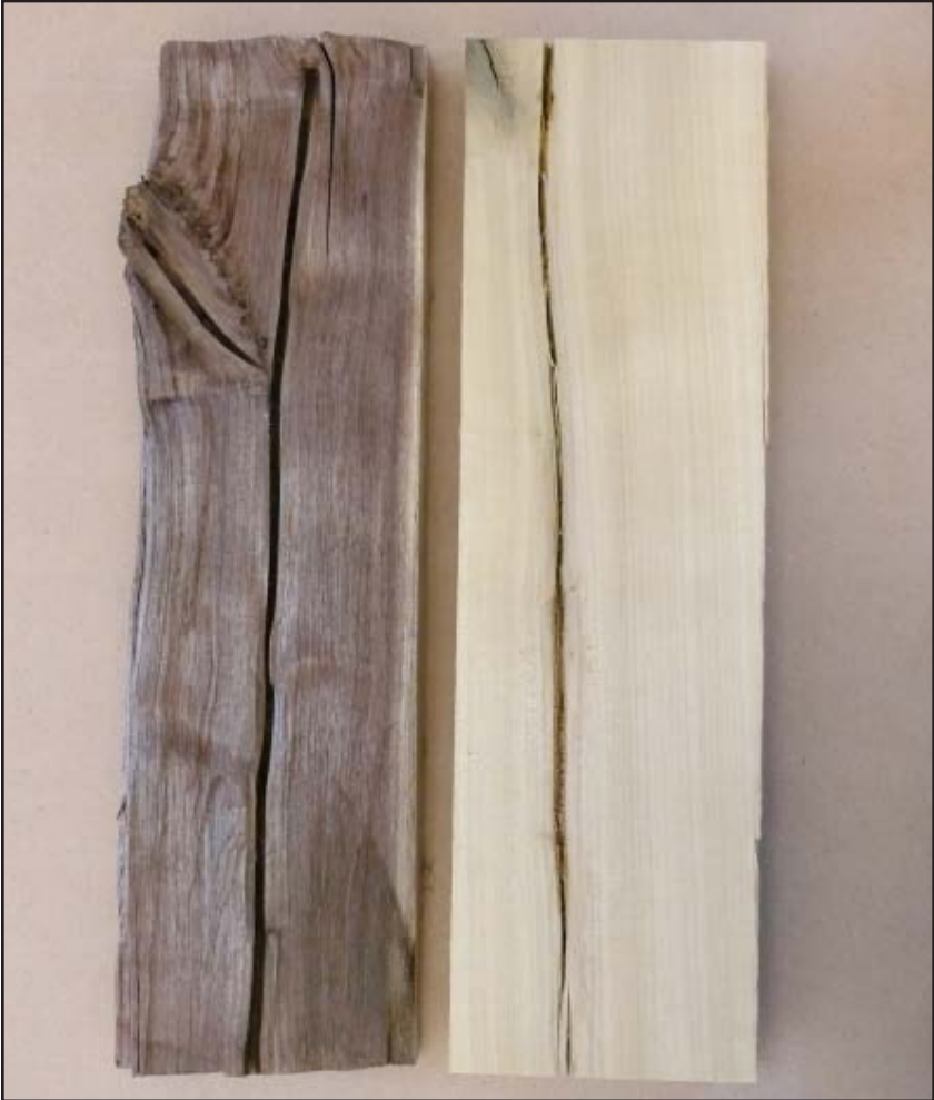
Figure 3-1. Examples of a large chambered pith in walnut (left) and a solid pith in yellow-poplar (right). Pith runs the entire length of the stem but, due to irregularities, it usually weaves in and out of a board.
