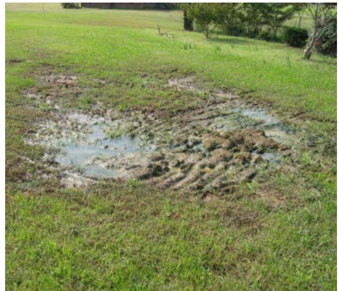
Figure 16. Septic systems are often forgotten until they have failed. A failing septic system (above) can leach toxic sewage into bodies of water, increase nutrient loads, make people and wildlife sick, become unsightly, and smell bad. It is much cheaper to maintain a septic system than pay for costly repairs. Photo by: Alamance County Environmental Health
