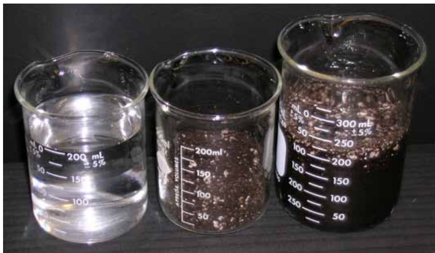
Figure 7. In the 1:2 dilution method, combine one part (by volume) of substrate with two parts (by volume) of distilled water.
