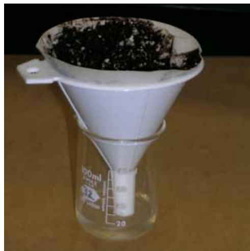
Figure 6. For the saturated media extract and 1:2 dilution methods, pour the samples into a clean funnel lined with filter paper or coffee filters to collect the extract.
