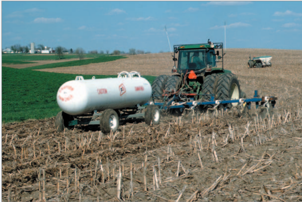
Figure 3.21. This implement is applying anhydrous ammonia on a field with corn residue cover. The white tank (“nurse tank”) contains ammonia under pressure. Photo provided by USDA-NRCS.
