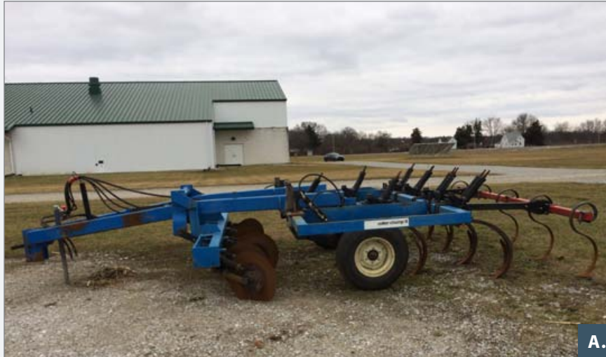
Figure 3.12. A. A chisel plow. The disk blades in front (left) cut through residue such as corn stalks and create a slice in the soil. The second and third units (behind tires) are the chisel plow shanks and shovels, four in the second unit and five in the third unit. They till about 10 inches deep. The last unit consists of S-shaped shanks and triangular shovels (sweeps) that smooth out the soil surface. B. A close-up taken from the other side of the implement shows details of the chisel shanks and shovels. These shovels are not twisted, so they bury less plant residue. C. Chisel plowing with a different implement. This one left little residue on the surface. 3.12C provided by Tom Bechman.
