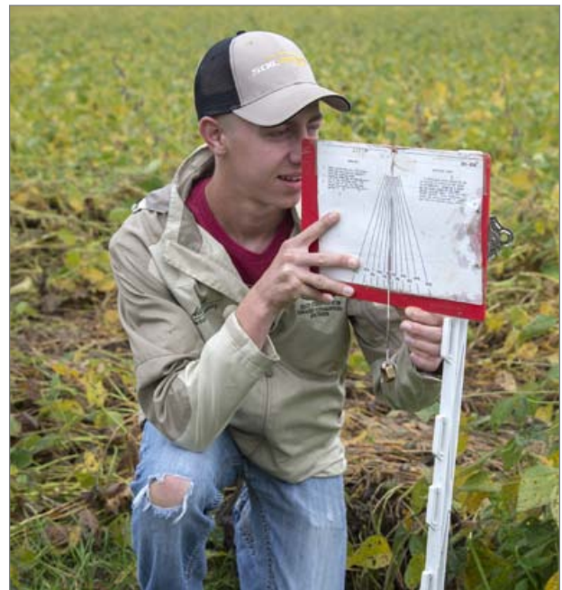
Figure 2.8. The contestant in this photo is measuring a slope with a slope finder (see page 148).
