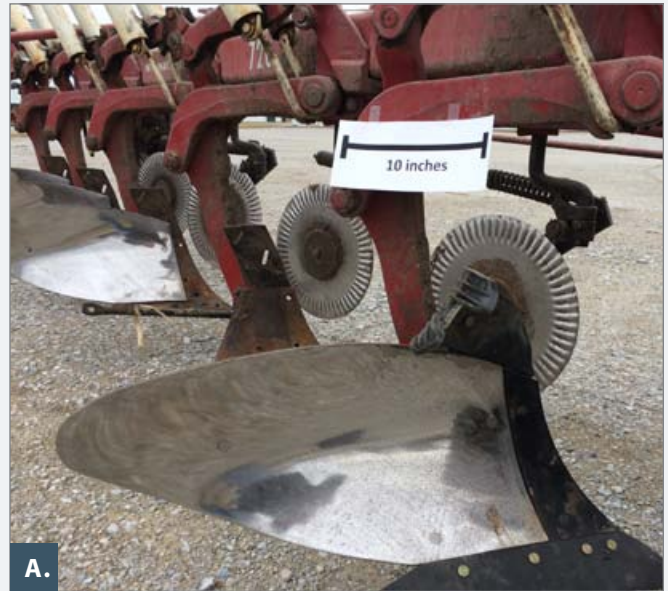
Figure 3.11. These photos show two views of moldboard plows. A. A moldboard plow out of the ground. The disk in front (far right) makes a shallow slit in the residue and soil surface. The shiny object is the plow. An important attribute is that soil does not stick to the metal surface of the plow (it “scours”). This implement has five units (a five-bottom plow). B. A four-bottom plow in action. It turns the soil completely over and buries almost all of the plant residue. Photo provided by Tiny Farm Blog.
