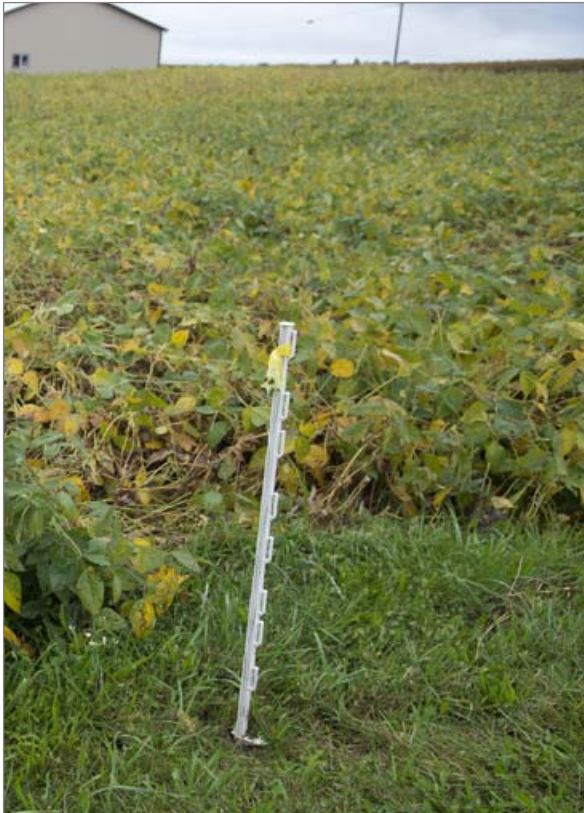
Figure 5.1. A small plastic fence post serves as a slope stake.
