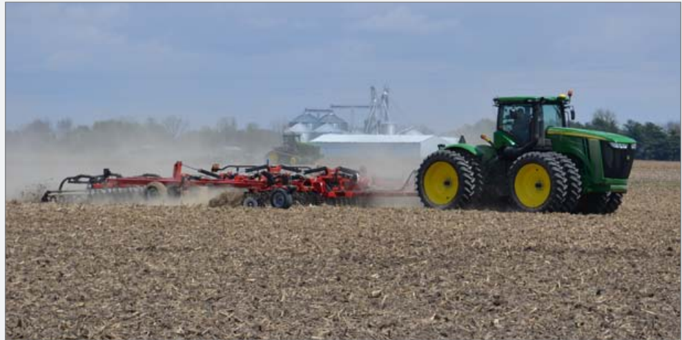
Figure 3.13. Using a disk/ field cultivator to prepare a field with corn residue for planting soybeans. Photo provided by Tom Bechman.
