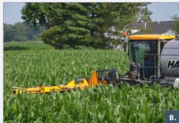
Figure 3.20. Applying liquid fertilizer to corn. A. This vehicle is applying fertilizer at the V-12 stage with a high-clearance sprayer. V-12 means that the corn plants have 12 leaves each. B. Applying nutrients to foliage with Y-drops, which are devices that place the N solution about 2 inches from the corn plant. Photos provided by Tom Bechman.
