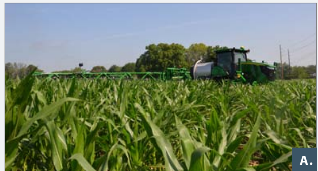
Figure 3.20. Applying liquid fertilizer to corn. A. This vehicle is applying fertilizer at the V-12 stage with a high-clearance sprayer. V-12 means that the corn plants have 12 leaves each. B. Applying nutrients to foliage with Y-drops, which are devices that place the N solution about 2 inches from the corn plant. Photos provided by Tom Bechman.
