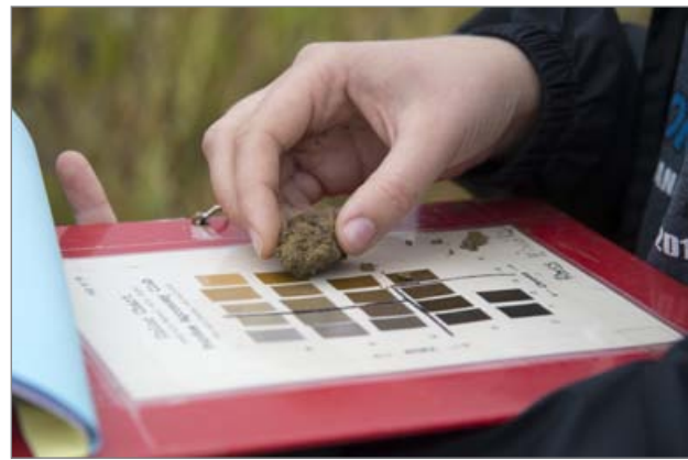
Figure 2.13. A contestant determines a soil's color using a Munsell color chart.
