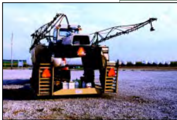
Pesticide application rig being transported on a trailer. Notice 2.5-gallon pesticide containers placed precariously near back of trailer where they could easily fall off and spill (above). The use of heavy machinery around power lines requires skill and caution (above right).
