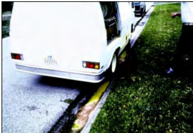
Work-site spill caused by broken hose
