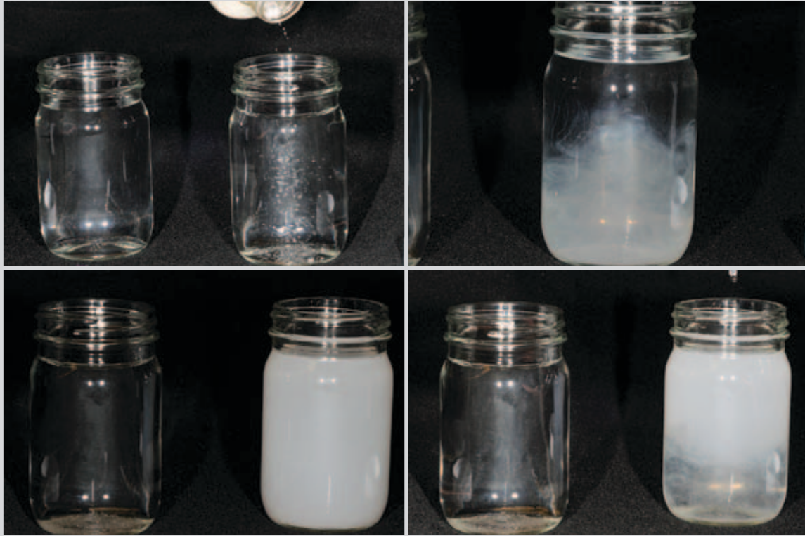
The bottle on the left (in each photo) contains distilled water with zero hardness; the bottle on the right contains hard water. A material that mimics glyphosate is added to both bottles of water. Notice that the water on the left remains clear, indicating the added product is in solution. The water on the right is cloudy, indicating that the calcium has bound to the glyphosate mimic.
