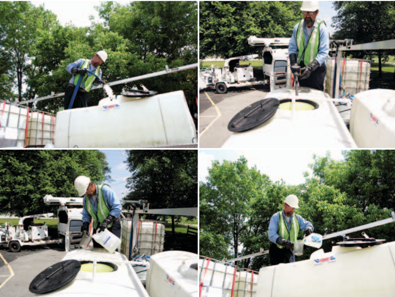
The use of water for application is nearly universal for all pesticide products. The tank is filled with water (top left); pesticide product is metered into the tank (top right); a spreader/sticker adjuvant is added to the mixture (bottom left); and a water conditioner is added to improve the quality of the water (bottom right).
