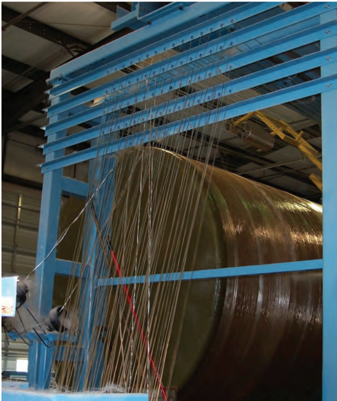
(Clockwise from top left) The manufacturer places a tank bottom on a mold (also called a mandrel). Next to the mold, spools of glass strand are lined up on racks. When the tank is built, glass strands are wrapped around the spinning mandrel. After that, the manufacturer applies the chop hoop layer, laying down “ropes” of glass that are made of about 60 strands each.
