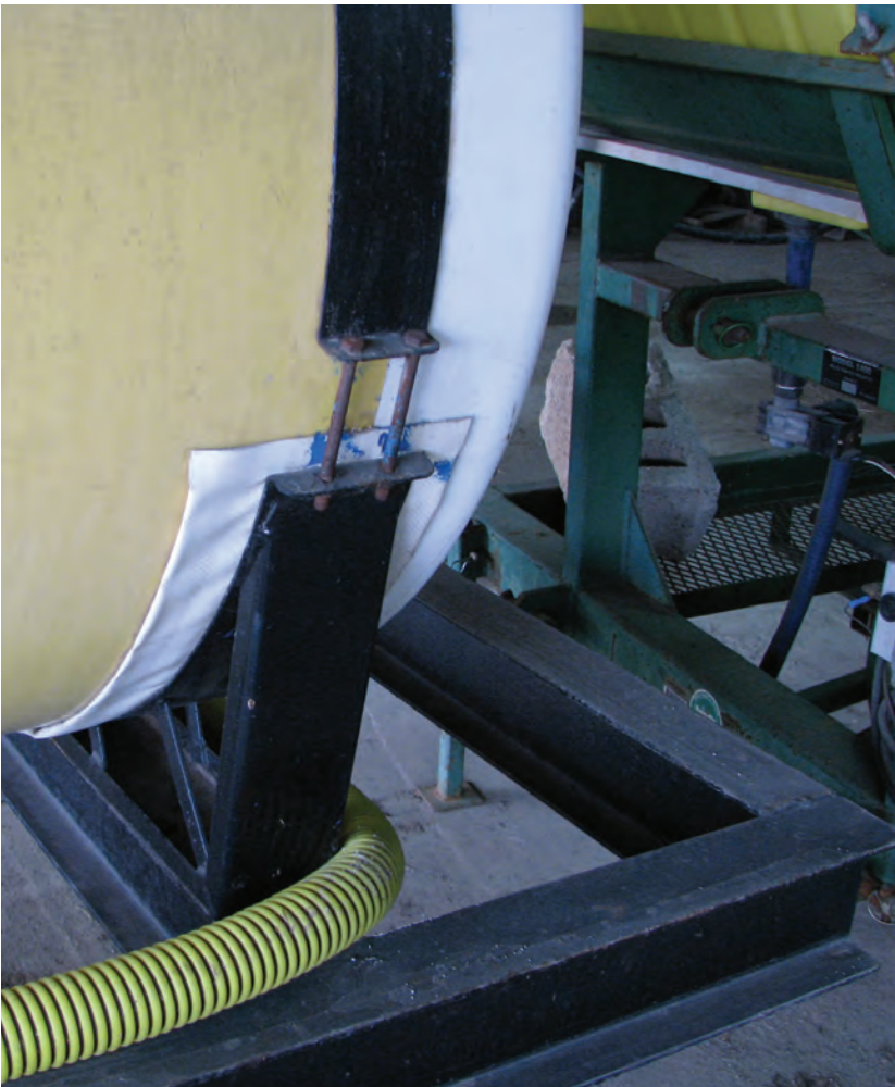
(Bottom left) A soft insert separates this tank from metal. (Bottom right) The soft insert for this tank fell out and the tank was damaged when it rubbed against the metal frame.
