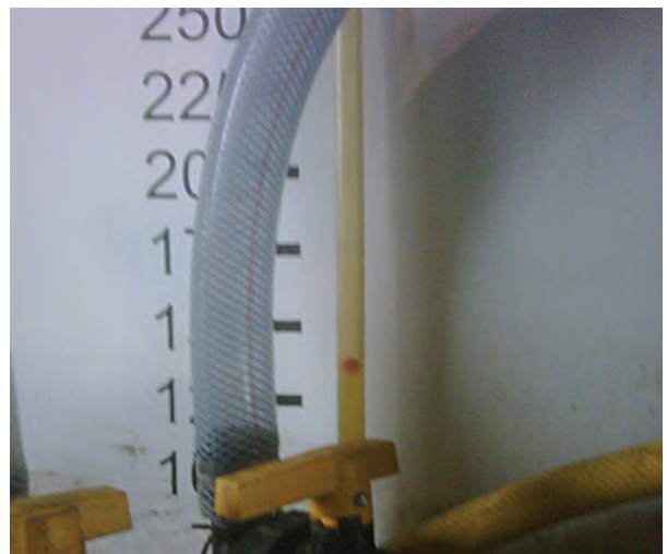
(Below left) A translucent area with graduated markings allow you to estimate a tank's contents. (Below right) The red ball floating in the liquid helps you gauge how much is left in the tank.
