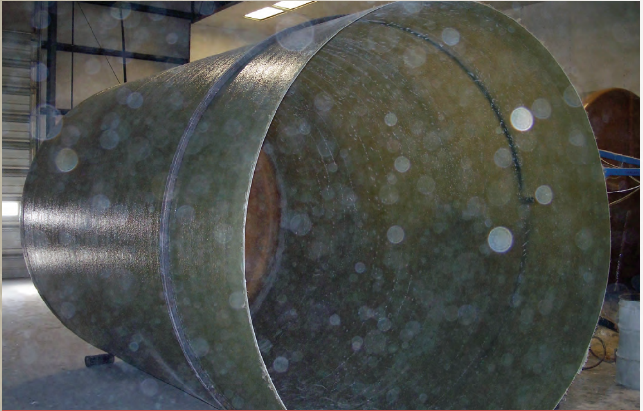
This fiberglass tank has been removed from its mold. A removable steel ring placed near the opening where the top will eventually be prevents the open end from collapsing.
