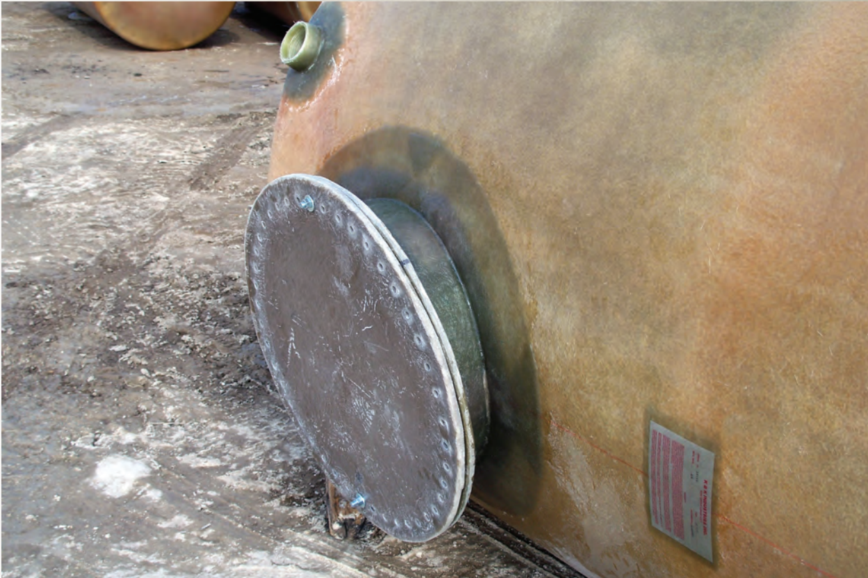
Once the tank is completed, the fiberglass seals the gap between the tank shell and flanged manway fitting. The darker circle in this image is a cosmetic effect from the use of different batches of resin.
