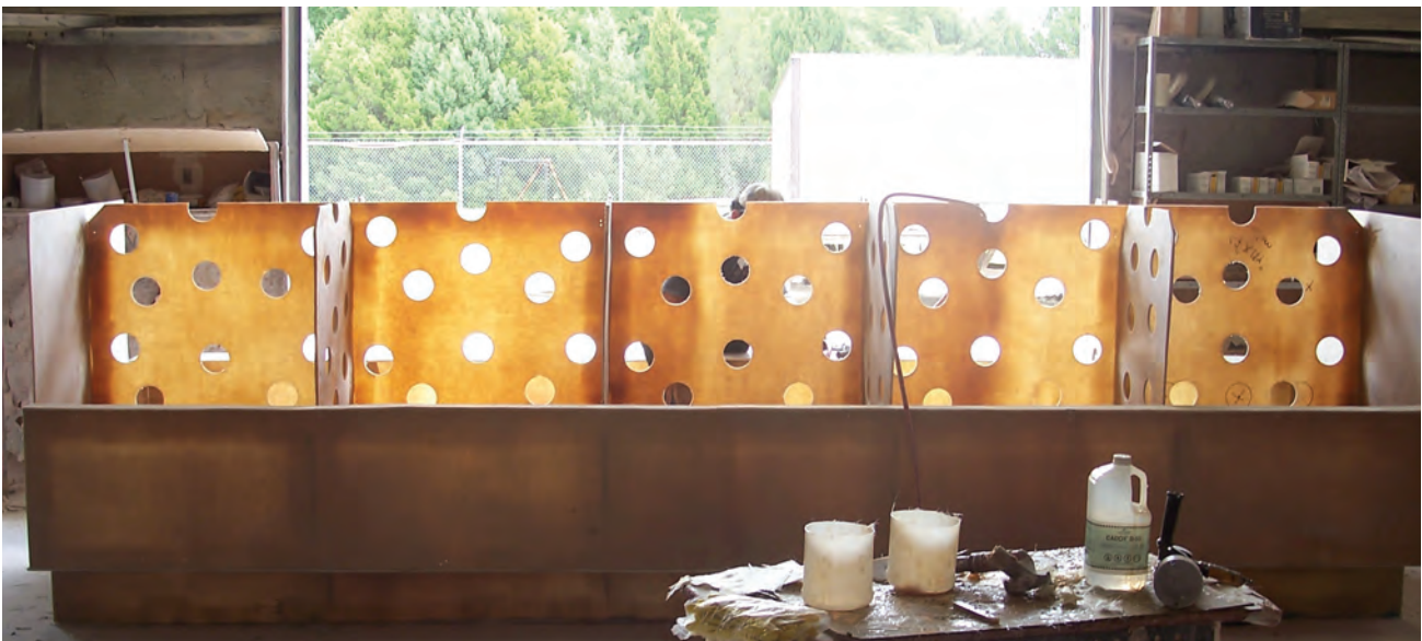
This vehicle-mounted tank is being outfitted with full-length and -width baffles.
