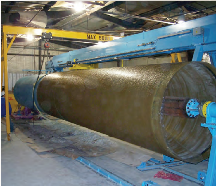
This brown fiberglass tank is newly formed and is being pulled off its blue mold. After the liner is removed, the tank will be cut to length and the top and bottom pieces will be put on.
