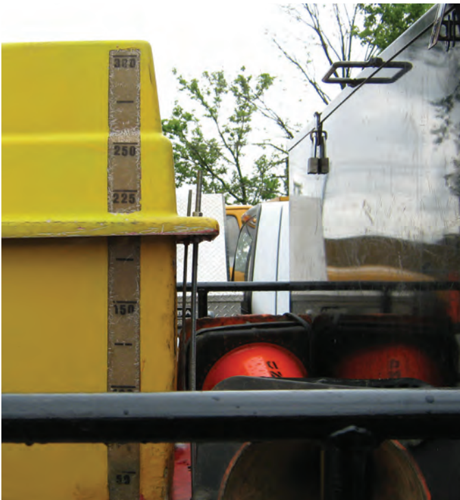
(Below left) A translucent area with graduated markings allow you to estimate a tank's contents. (Below right) The red ball floating in the liquid helps you gauge how much is left in the tank.
