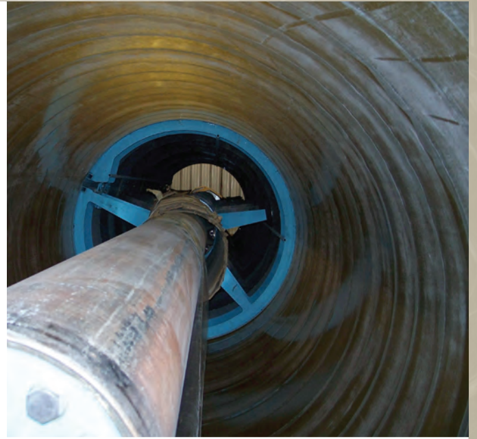
This brown fiberglass tank is newly formed and is being pulled off its blue mold. After the liner is removed, the tank will be cut to length and the top and bottom pieces will be put on.
