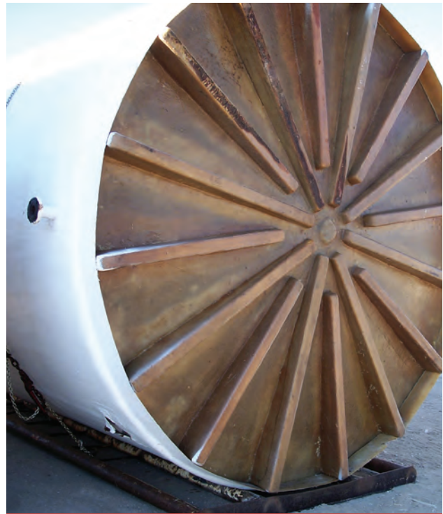
The underside of this dish-bottom tank has a 3- to 6-inch slope to the center, which allows its contents to be fully drained.
