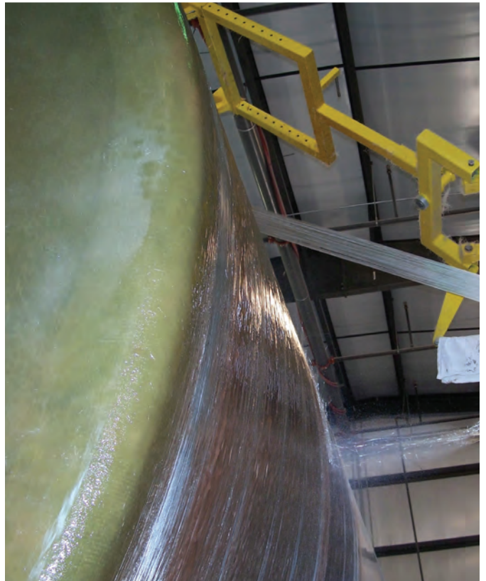
(Clockwise from top left) The manufacturer places a tank bottom on a mold (also called a mandrel). Next to the mold, spools of glass strand are lined up on racks. When the tank is built, glass strands are wrapped around the spinning mandrel. After that, the manufacturer applies the chop hoop layer, laying down “ropes” of glass that are made of about 60 strands each.
