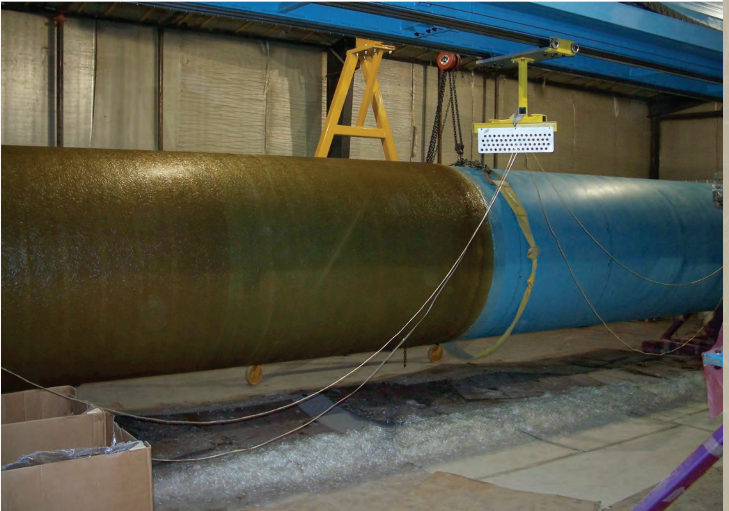
This brown fiberglass tank is newly formed and is being pulled off its blue mold. After the liner is removed, the tank will be cut to length and the top and bottom pieces will be put on.
