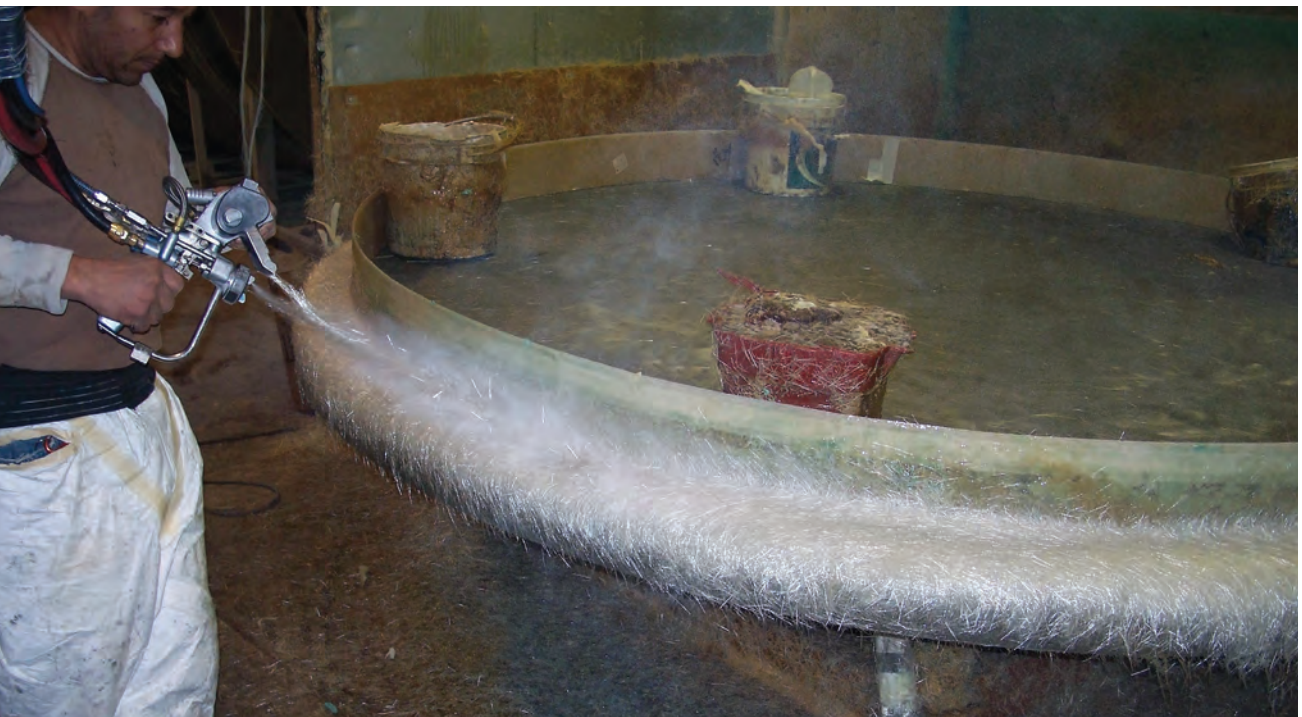
This chopper gun mixes resin with extruded glass as it leaves the gun.
