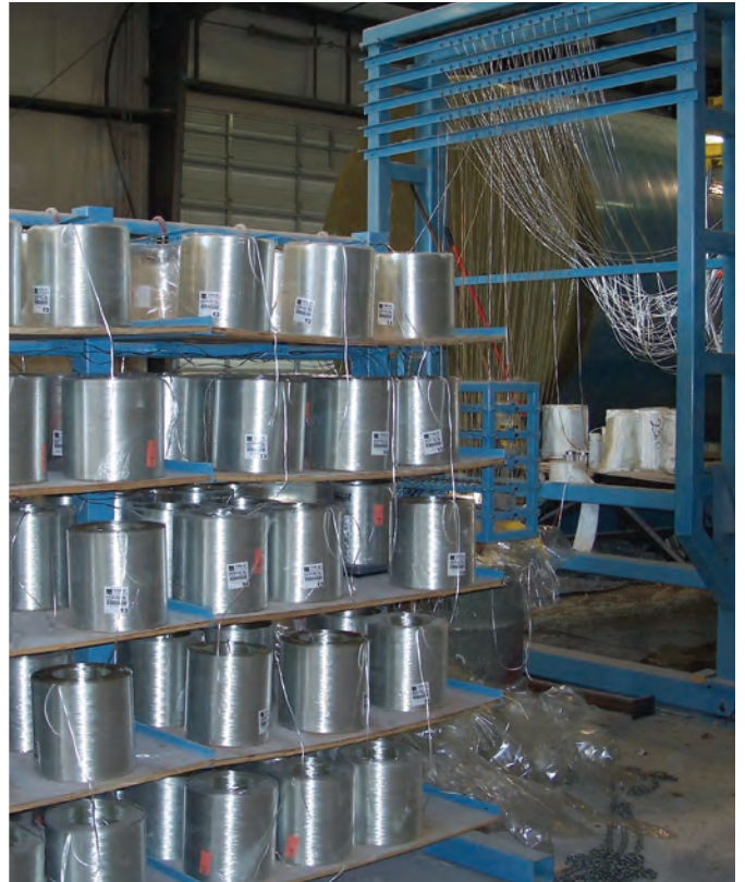
(Clockwise from top left) The manufacturer places a tank bottom on a mold (also called a mandrel). Next to the mold, spools of glass strand are lined up on racks. When the tank is built, glass strands are wrapped around the spinning mandrel. After that, the manufacturer applies the chop hoop layer, laying down “ropes” of glass that are made of about 60 strands each.
