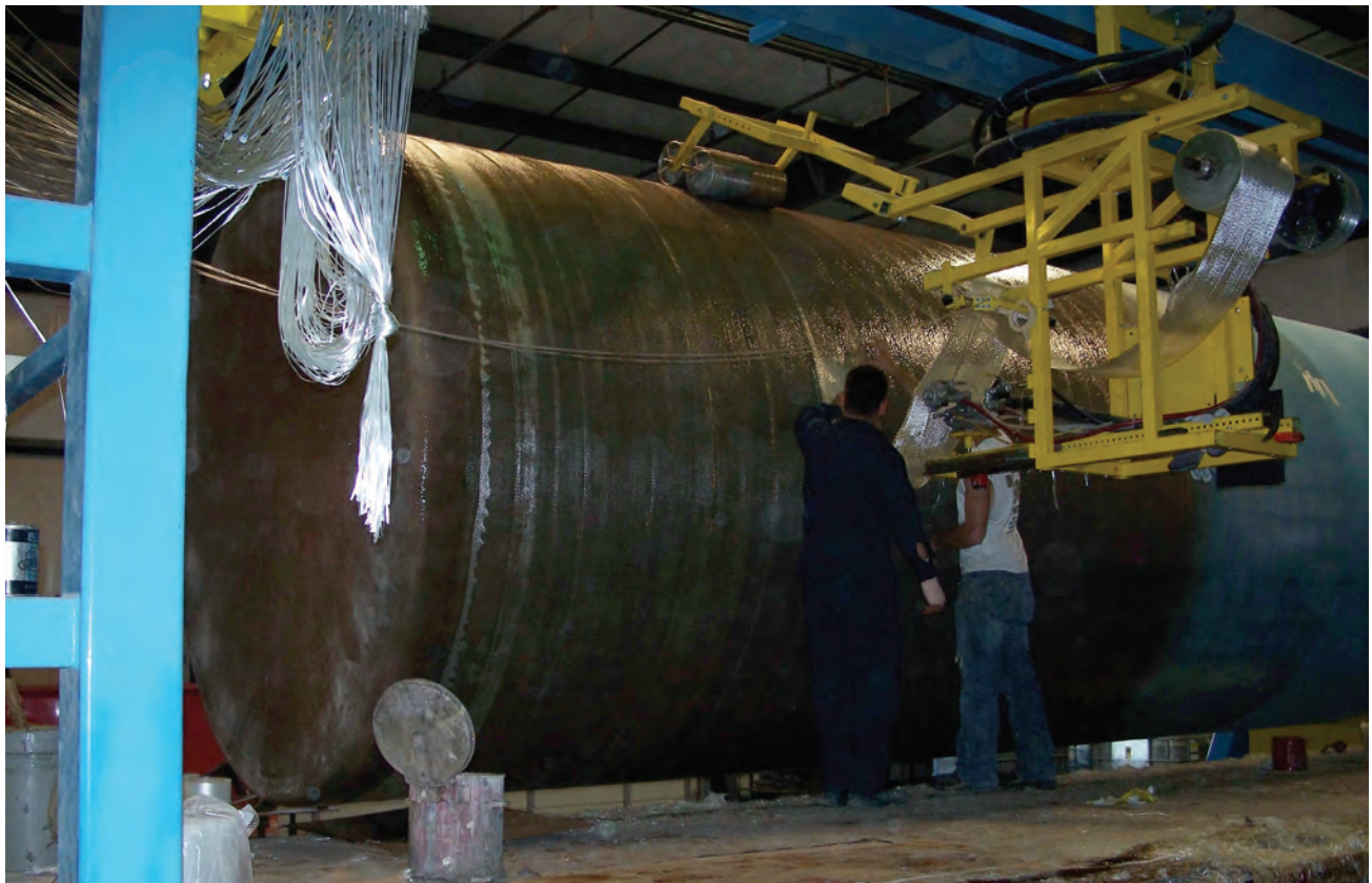
In this photo, the blue cylinder is the mold and the fiberglass tank being formed is brown. When complete, this tank will measure 10 feet wide, 15 feet tall, and hold 8,800 gallons.
