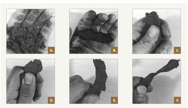
Figure 5. The casts of different soil samples when you squeeze them in your hand to determine soil texture group. A: a sandy texture. B and C: moderately sandy. D: medium. E: moderately clayey. F. clayey.
