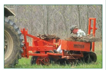
**Figure 7.** A mechanical tree planter suitable for planting large bare-root seedlings. (Photo courtesy of Ron Rathfon)
