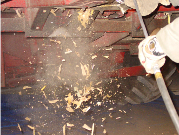
Figure 5. Using compressed air to clean out the feederhouse.
