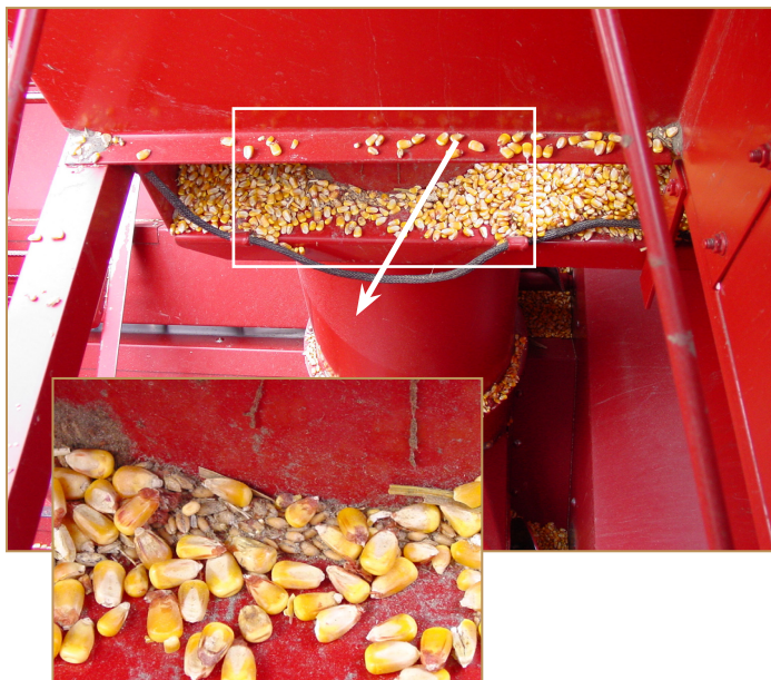
Figure 3. Ledge in grain tank after approximately 6,000 bushels of corn harvested. Note residue from prior wheat harvest.
