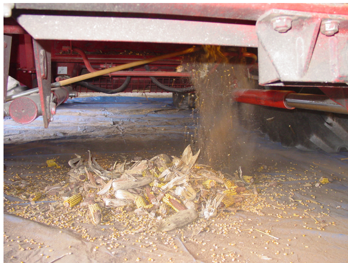
Figure 4. Emptying of the rock trap.
