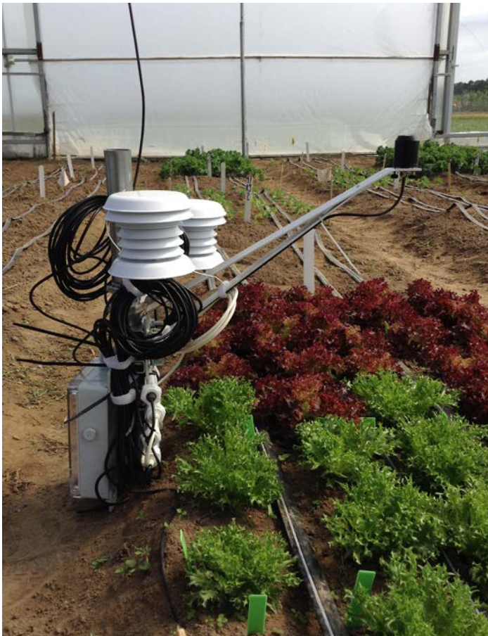
Figure 15. The metal support extending over the lettuce supports a light (PAR) sensor (the black cylindrical object). The other sensors and nearby objects are below the level of the light sensor so they will not shade it. (Photo by E. Bluhm.)
