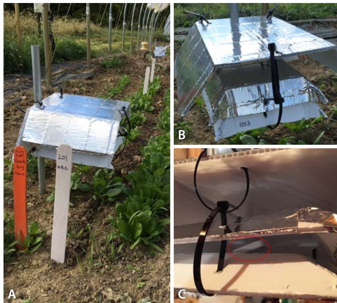
Figure 14. A. Homemade radiation shield in use in a high tunnel. B. Close-up of radiation shield shown in A. C. Close-up of radiation shield showing location of temperature sensor between bottom and second layer of shield.
