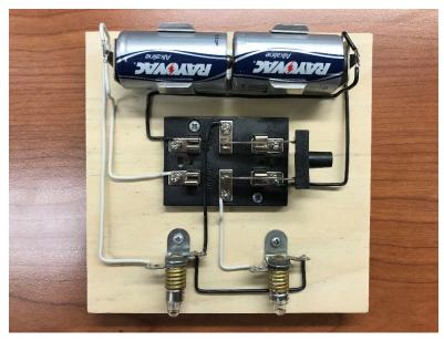
A double-pole-double-throw switch may be used to connect two electric loads in series or in parallel. For example:
