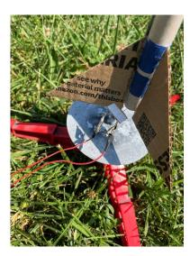
Make sure to use fresh batteries and that your clips do not touch each other or any metal launch pad components. Don't twist the igniter wires!
