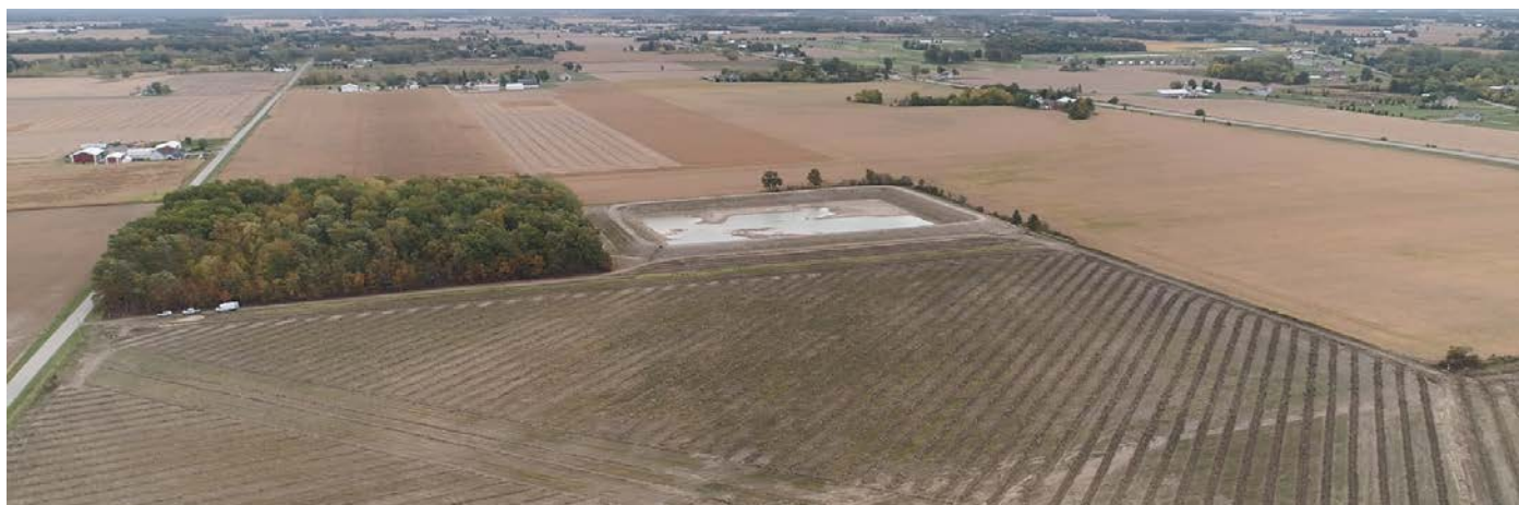
Figure 6. This reservoir has been designed and sized appropriately to capture water from the tile drained field and supply sufficient water as subirrigation during the growing season.
