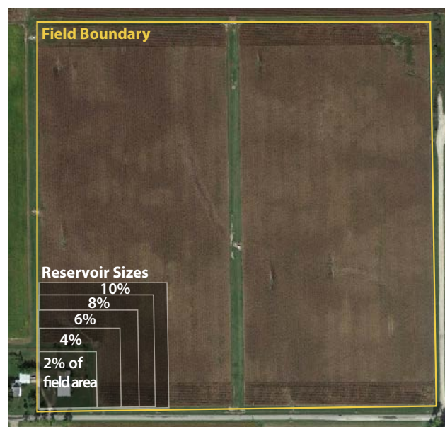
Figure 3. This case study evaluated a range of reservoir sizes representing between 2 percent and 10 percent of the overall field area (assumed average depth of 10 feet).
