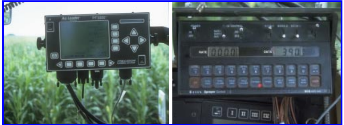
Figure 3. Site-specific application system display unit (on the left) and an electronic application controller.
