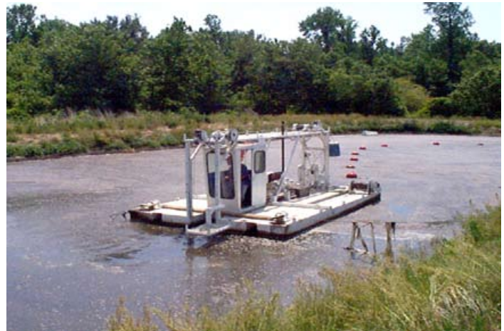
Figure 2. Pumping dredge operating in a lagoon in North Carolina.
