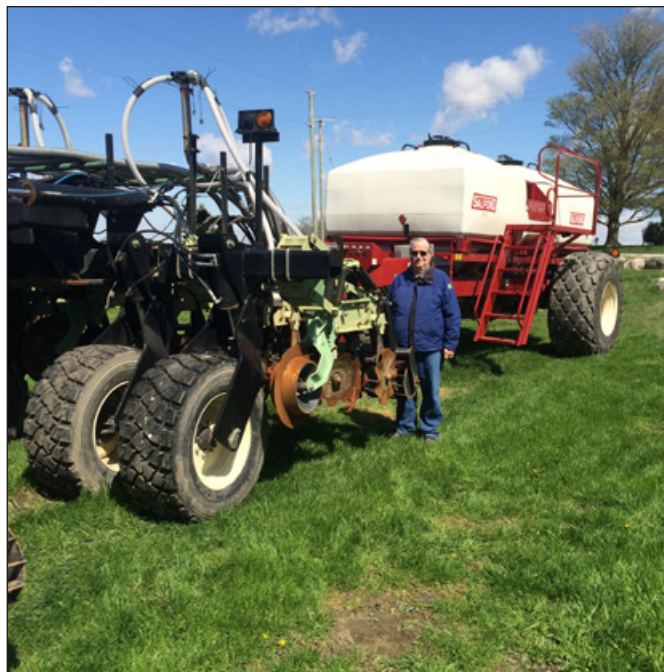
Figure 7. You can incorporate fertilizer with shanks, coulters, or knives. This producer in Frankton, Indiana, is using a deep-banded strip-till system. Incorporation decreases DP loss in surface runoff. Photo by Tony Vyn.
