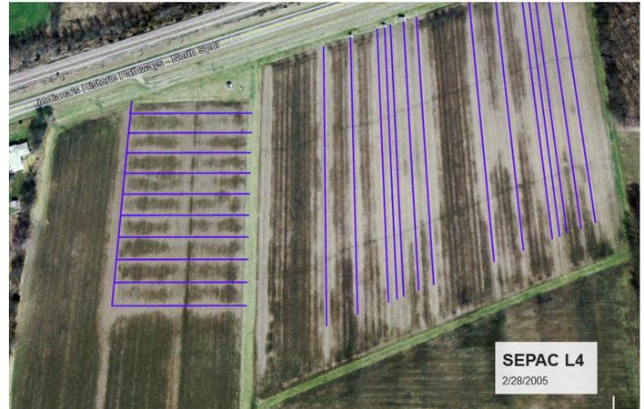
Photo 3. Aerial image of drainage field, with drain lines superimposed on the image. The lighter-colored soil over the drainlines clearly shows the impact of the drains on drying the soil faster than where drains are not present. Note the darker areas in the right-hand side of the field, correspond to the undrained control (compare to Fig. 1 for field design).
