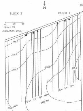
Figure 1. SEPAC drainage spacing field layout.
