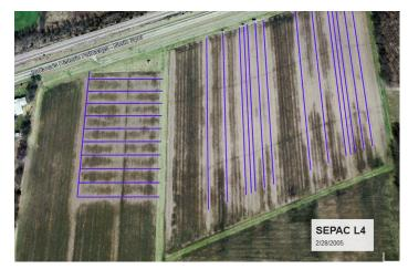
Photo 3. Aerial image of drainage field, with drain lines superimposed on the image. The lighter-colored soil over the drainlines clearly shows the impact of the drains on drying the soil faster than where drains are not present. Note the darker areas in the right-hand side of the field, correspond to the undrained control (compare to Fig. 1 for field design).
