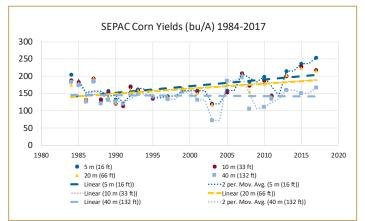
Figure 5. When looking at the corn yield trend over time, from the first to most recent corn year, the trends for the three drain spacings are similar to general corn yield trends reflecting improvements in genetics and other practices, while the undrained control has remained flat or even decreased slightly.
