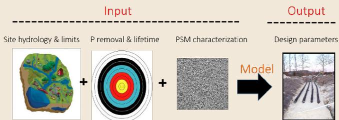
Structures are constructed based on a desired P removal goal and lifetime in accordance with site conditions (flow rate and DP concentration). For example, a 10yr-40% goal means that the structure is designed for removing 40% of all the DP that flows into a structure over 10 years. For details on P removal structures and how to gather inputs, see [Penn, C.J., and J.M. Bowen. 2017. Design and construction of P removal structures for improving water quality. Springer Publishing.](#)
