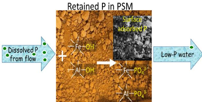
Example of a P removal structure and components, specifically a subsurface tile drain P filter using iron and aluminum metal hydroxides.
