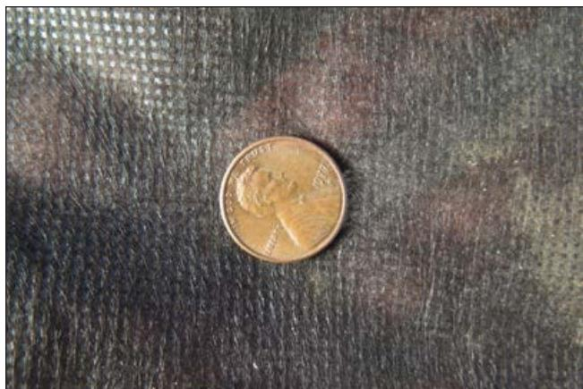
**Figure 9.** Black landscape fabric that lies underneath the white ground cover shown in Figure 8. The landscape fabric keeps the white ground cover relatively clean.
