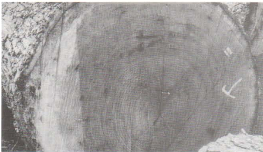
Figure 18. Isolated spots of mineral stain in northern red oak.
