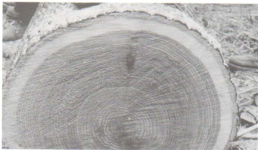
Figure 17B. Defect associated with "bars" on red oak log.
