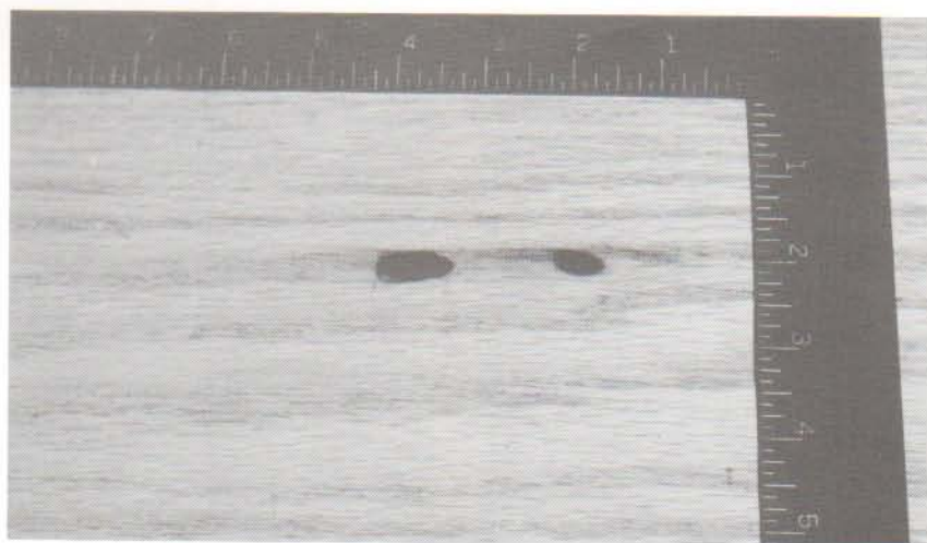
Figure 16C. Typical borer damage in red oak veneer.
