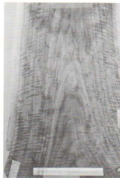
Figure 12. This walnut veneer is muddy and lacks uniformity in color. It also has a curly grain pattern or flare, which is often objectionable in most applications. However, if the wood is uniformly figured and the flitch is large enough for a particular application, it may have exceptional value.
