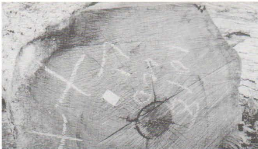
Figure 15. Stump worms and associated stain in white oak caused by worm from livestock, fir, or mechanical damage. These defects appear mostly in the upper and left portions of the log.
