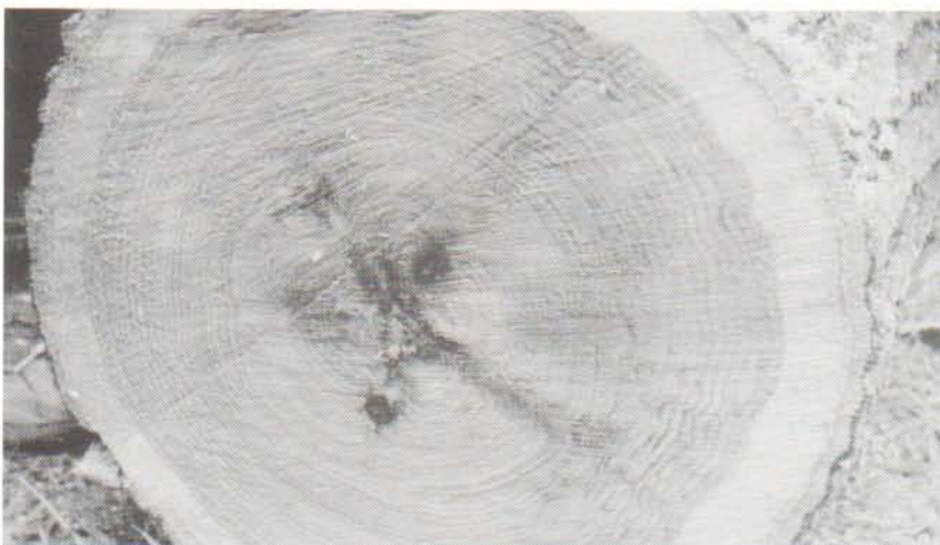
Figure 19. Mineral stain following the annual rings in northern red oak.
