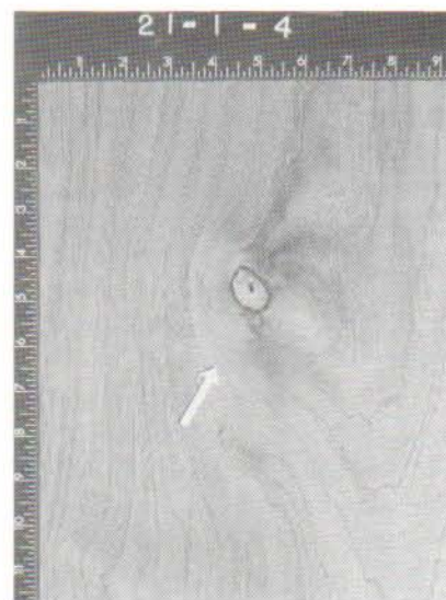
Figure 7D. The entire cross section of the knot appears at a depth of 4 inches.
