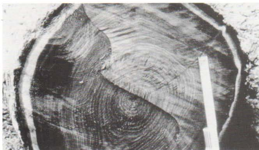
Figure 10A. Pin knot on the end of the log shown in 10B. The knot appears as a trace or streak from near the center of the log and terminates in a bump in the white sapwood.
