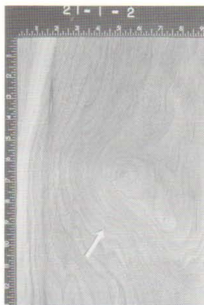
Figure 7B. Grain distortions resulting from the barely conspicuous defect in Figure 7A are visible at a depth of 3 inches. Light-colored sapwood, which is discarded by most veneer users, is visible on the left side of the photo. The dark streak or mineral stain in the upper left is also considered a defect in high-quality veneer.
