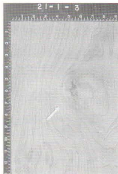
Figure 7C. The limb stub or knot becomes visible at 3 1/2 inches.
