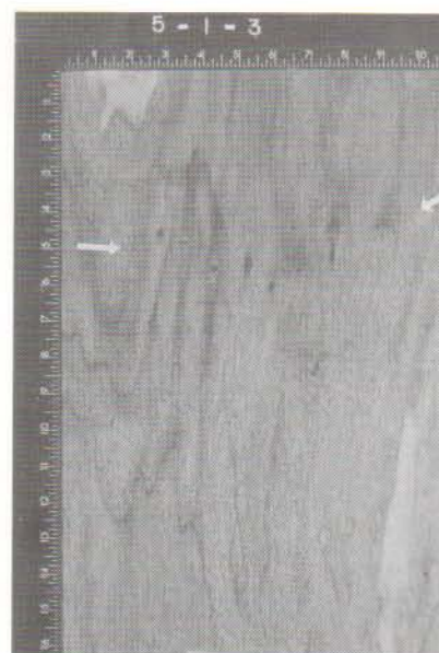
Figure 11C. Several peck marks and associated stain from the log shown in 11B.
