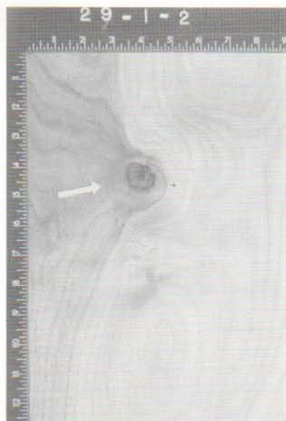
Figure 6C. The entire cross section of the knot became visible 3 inches below the surface.
