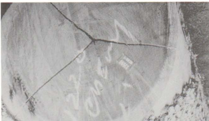
Figure 24A. Gum spots appear as small dark spots on the end of a cherry log.
