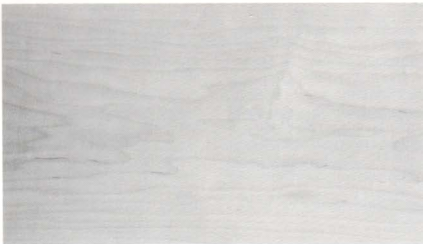
Figure 23. Sugar streaks or flecks in sugar maple veneer.
