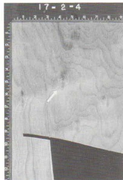
Figure 9B. Pin knots were located 3 1/10 inches beneath the log surface. However, the knots were first visible just beneath the surface.
