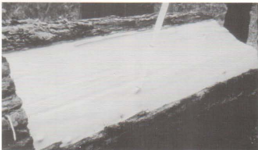
Figure 10B. Pin knots on the surface of a walnut log.
