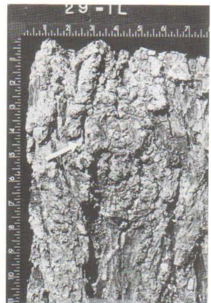
Figure 6A. A conspicuously overgrown limb stub resulting in a well-defined break in the bark of black walnut.
