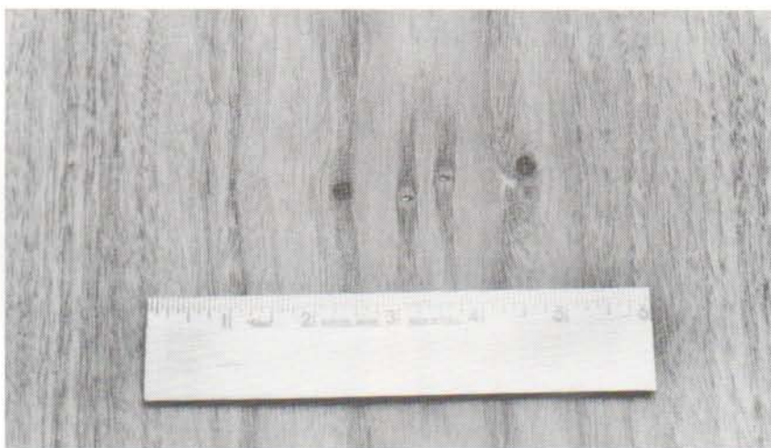
Figure 10. Worm holes and associated stain (center two) in walnut.
