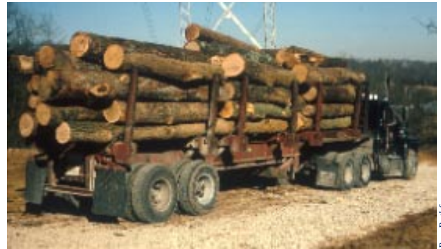
The judicious use of gravel can prevent unsightly rutting and erosion and prevent log trucks from tracking mud on to public roads.
