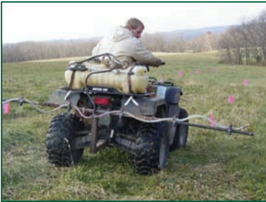
Figure 8. ATV with mounted boom sprayer can be very useful for small planting areas or uneven terrain. (Photo courtesy of Ron Rathfon)
