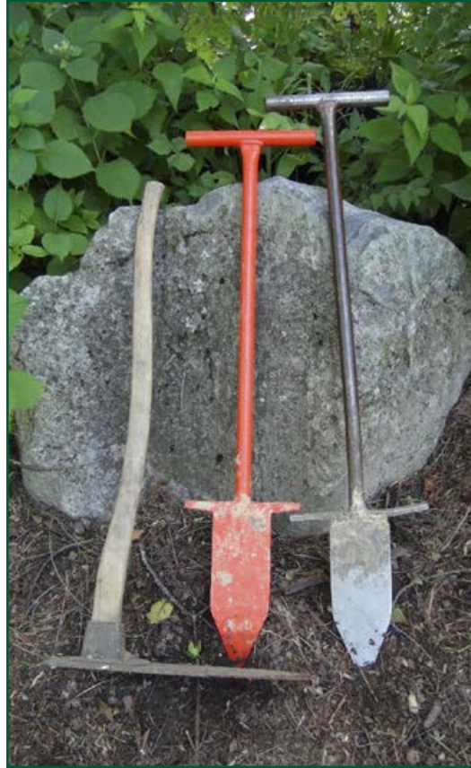
Figure 4. Some tools for hand-planting hardwood seedlings (left to right: Hoedad, KBC bar, and a shop-built tree planting bar). Photo by Lenny Farlee
