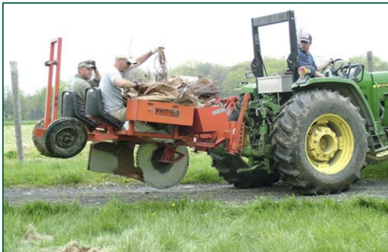
Figure 7. A mechanical tree planter suitable for planting large bare-root seedlings. Photo courtesy of Lenny Farlee
