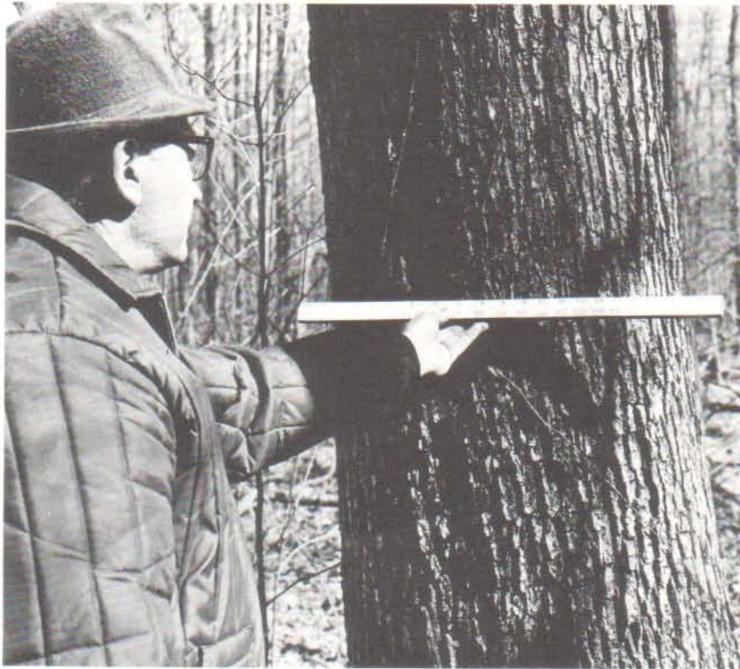
Figure 3. Tree diameters are measured 4.5 feet above the ground, a convenient and standard point of measurement.
