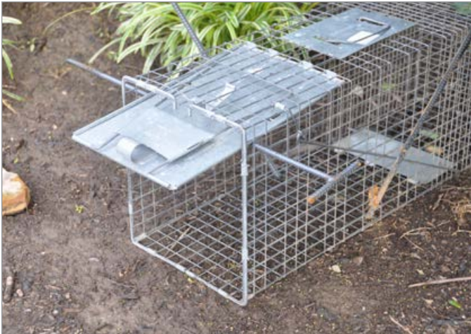
Figure 7. Using a stake or similar device to hold the trap door open is helpful when pre-baiting a trap or releasing a captured animal.
