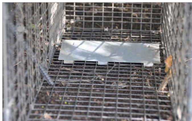
Figure 2. View of the trap treadle (sometimes called a pan). Make sure the space under the treadle is clear of sticks, rocks and other debris that may interfere with trap function.
