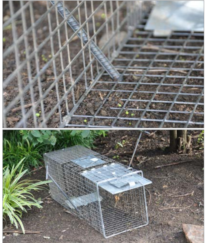
Figure 4. A metal rod pushed through both the side and base of a box trap (top). Staking a trap on both sides (bottom) in this manner will prevent trap rolling.
