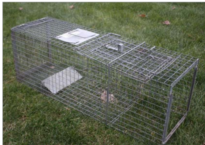
Figure 3. Specialty traps or trap accessories can be helpful in certain situations. For catching animals inhabiting burrows, a nose cone changes the position of the entry to the bottom of the trap. Since the nose cone extends beyond the door, the trap with nose cone assembly can be placed adjacent to a building or wall over a burrow entrance. Note that the sliding end door is removed on the pictured trap.
