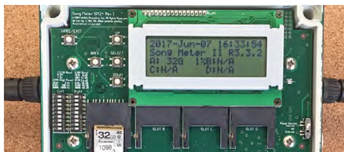
Figure 10.3. Turn the Song Meter on by moving the small power selection switch to the internal position.
