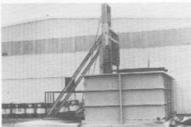
Figure 7. Dip tank for bulk piled bundles of lumber.
