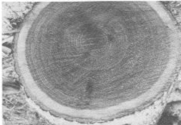
Figure 1. Large sapwood band on southern oak log (A) as compared to narrow band on northern oak log (B).
