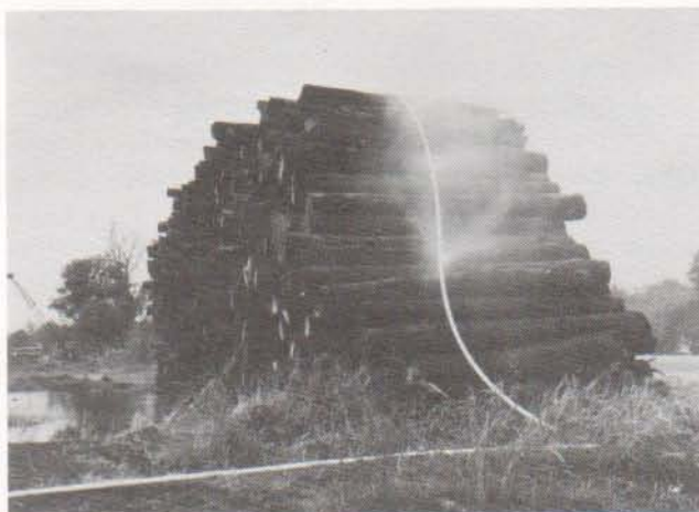
Figure 3. Water sprinkler system used to prevent log stain.
