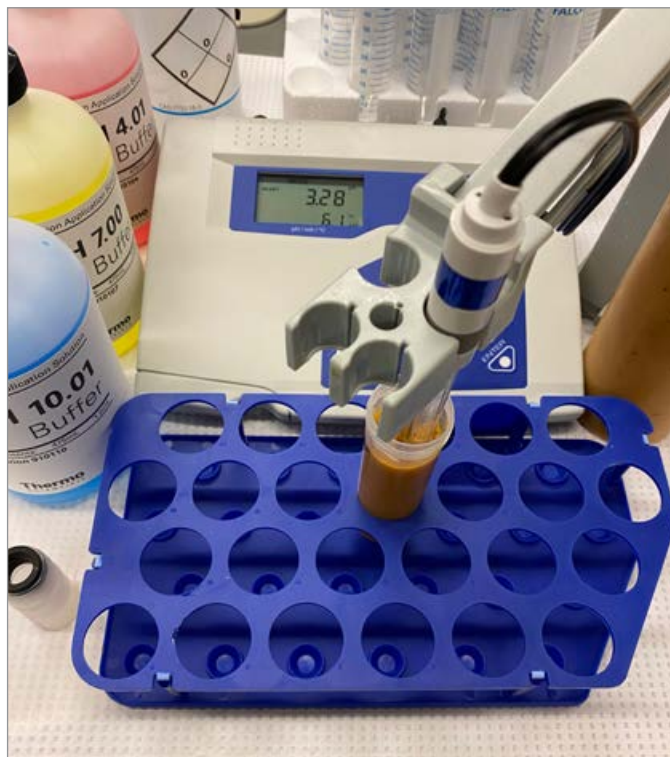
Figure 1. Measuring pH of a product with a pH probe.
