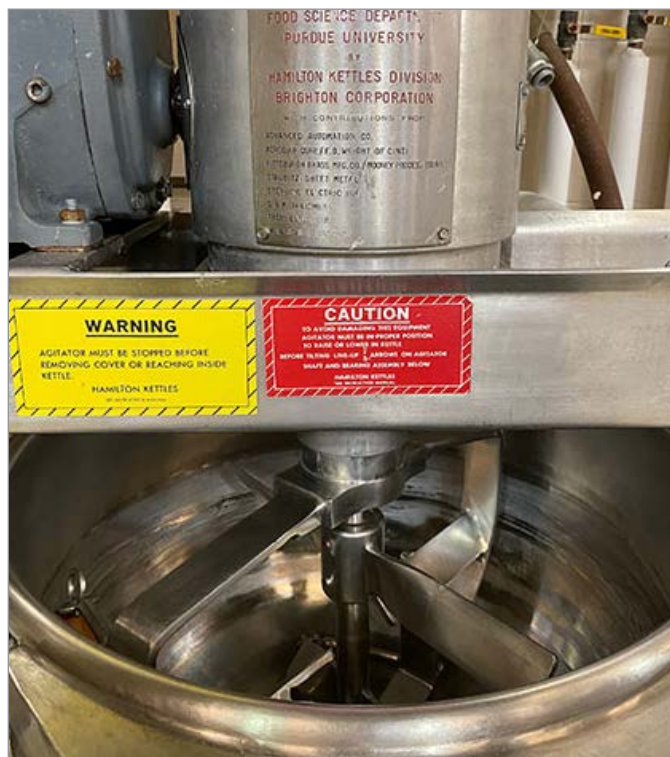
Figure 2. Steam jacketed kettle with a mixer to stir the product while cooking and holding for specified time and temperature.
