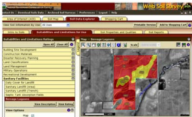
Figure 3. Illustration of soil suitability for a sewage lagoon. The red color indicates poor suitability and the yellow indicates moderate suitability.
