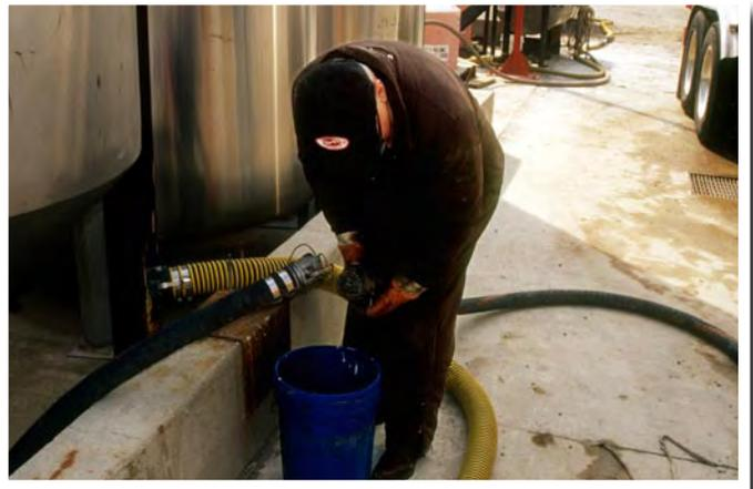
A pesticide manufacturer's driver uses a bucket to make sure that not a single drop of pesticide is spilled on the cement as he fills this bulk tank.
