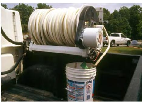
A bucket is used to collect any materials that are released from the nozzle (above).
