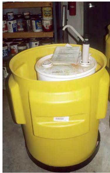
The bottom cut off of a large vinyl holding tank is used for containment (right). Although the picture doesn't show it, the cement floor has a large crack in it, making containment extremely important in this particular case.
