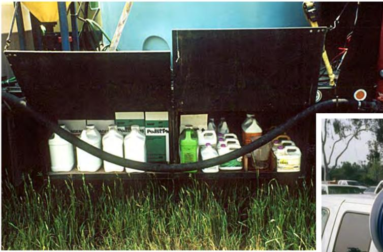
Pesticides are stored in a cabinet permanently mounted on a truck (above) and backpack sprayers are locked securely onto a transport unit installed in the bed of a truck (right).
