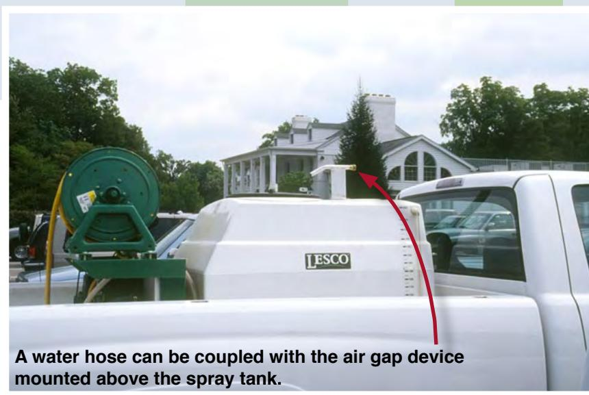
**A water hose can be coupled with the air gap device mounted above the spray tank.**
