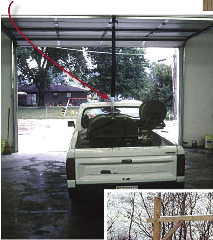
The operator must hold the hose to fill the tank. Spills enter the floor drain and are contained in a permanently sealed cement basin.
