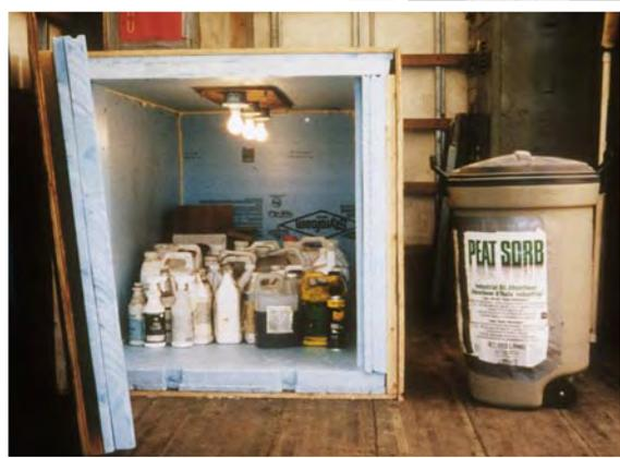
These photos show an insulated storage box, in an unheated building, that has three light bulbs inside to keep its contents from freezing.
