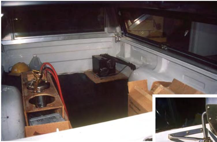
A wooden box is used to transport chemicals. A switch inside the cab directs heat from the radiator to the truck bed to keep chemicals from freezing.
