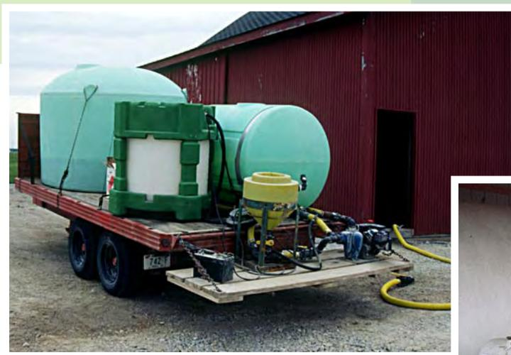
The water tank mounted on the trailer above is filled directly from a well. The water used to fill the sprayer comes directly from the tank, not the well.
