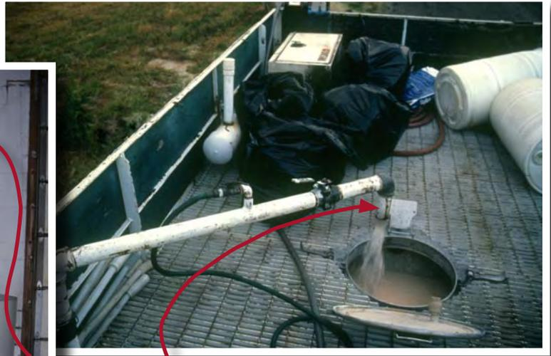
The water pipe in each example is suspended in mid air, leaving an air gap between it and the fill tank.
