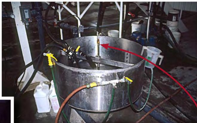
The tank above has been modified with a rinse jet that fits into the opening of a plastic jug; the rinsate drains directly into the spray tank.
