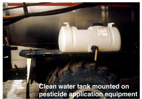
Clean water tank mounted on pesticide application equipment
