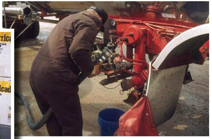
The common bucket provides simple but effective containment for leaks and drips.
