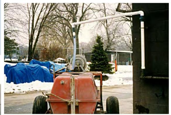
A "swing arm" elevates the hose above the tank in each of these examples.
