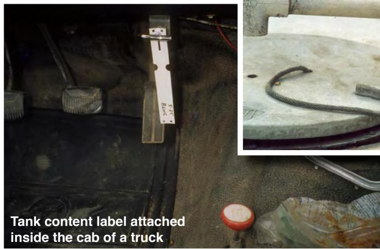
Tank content label attached inside the cab of a truck
