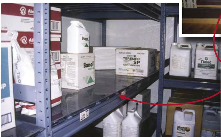
These photos show pesticides stored on trays with raised edges to contain any spills or leaks that might occur. The all-metal shelving unit (left) is a better choice than the metal/wood combination shelving (above); but, even so, the pesticides are "contained" on a tray.
