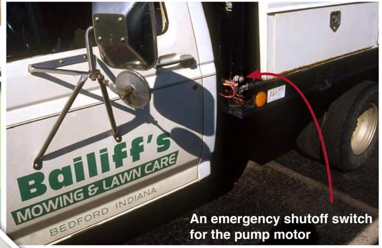
An emergency shutoff switch for the pump motor
