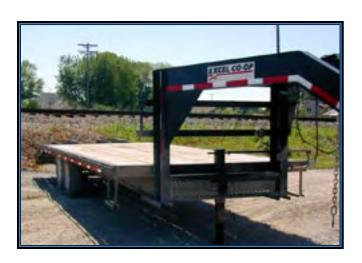
ings (GVWRs) greater than 10,000 pounds and widths of 80 inches or more must be marked with retroreflective tape. The tape must cover at least 50 percent of the length of each side of the trailer and be evenly distributed across the length.
