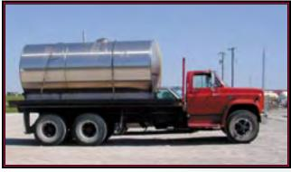
Is the tank capacity more than 119 gallons? Will it be used to transport hazardous materials? If yes to both questions, the vehicle and cargo are subject to DOT placarding regulations.
