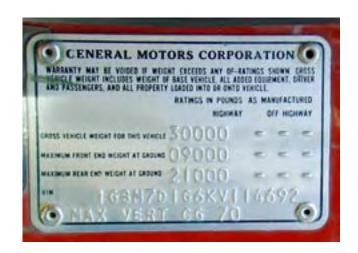
behind the driver on a panel mounted to the cab. The GVWR represents the maximum loaded weight of the vehicle as certified by the manufacturer; i.e., the maximum weight, including the vehicle itself, that the power unit or trailer can safely carry. The GVWR takes into consideration the suspension, tires, frame, and overall manufactured design strength of the vehicle.
