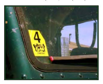
CVSA stickers are color-coded. Based on the color, the year, and the corner removed, officers can determine when a Level 1 inspection was conducted on a given vehicle. Vehicles displaying current CVSA stickers generally are not re-inspected unless there is an obvious driver violation or a noticeable defect in the vehicle or its cargo.
