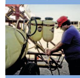
Closed-system transfer systems reduce exposure potential.
