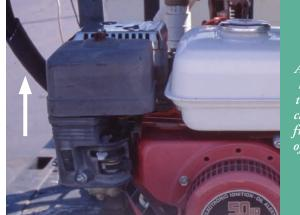
Another hose helps shield the pressurecarrying hose from the heat of the engine.
