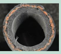
Hoses can wear from the inside, out. Proper hose inspection includes hose interiors and exteriors. If the tube cover separates from the inner hose, it is time to replace the hose.
