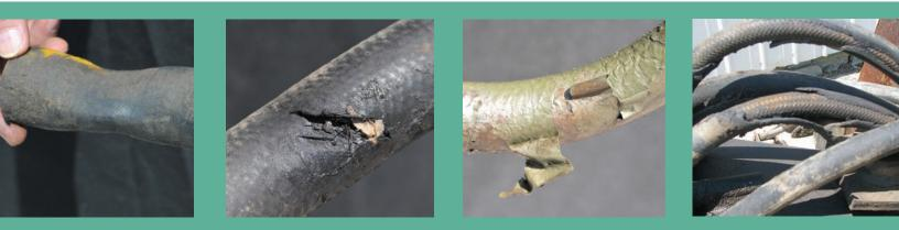
When oil or grease remain on a hose, it can create soft spots that weaken a hose's integrity.
