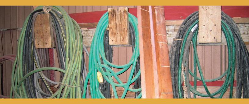
When handling chemical hoses, always wear the personal protective equipment required by chemical labels. Before removing hoses, make sure they are completely purged. And when replacing any hose, make sure to save any liquid it contains — plan ahead to catch the liquid so it does not spill in the shop or on the ground.
