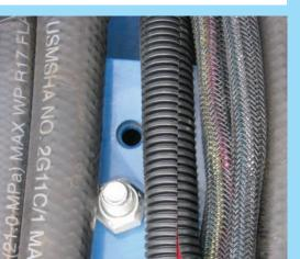
(Above) The hose on the left is not protected and rubbing against a metal bolt, which and can cause it to break down prematurely.
