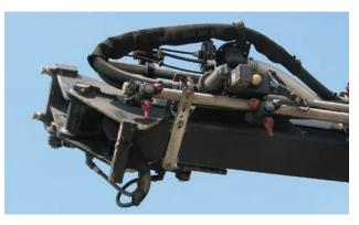
Improperly installed hoses can kink and fail.
