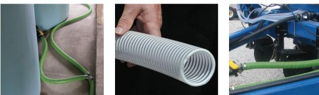
pump. Suction hoses fail when pumps create more vacuum — more suction — than the hose can resist. When this happens, the hose collapses.
