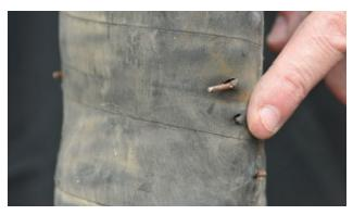
Kinking can permanently pinch the wire braid in hoses.
