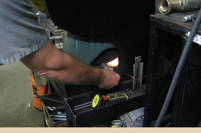
Cutting hoses requires the right tools. Don't forget that hose fittings require extra length — so account for fittings when measuring.
