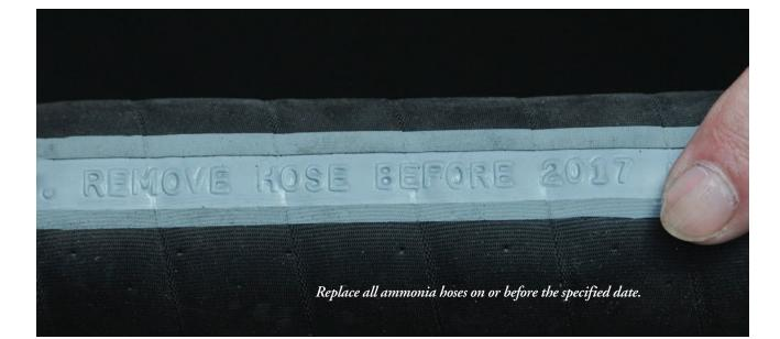
These high-performance hoses will frequently be stamped with the manufacturing date, manufacturer's name, working pressure, and bursting pressure. In some cases, manufacturers will recommend when to replace hoses.
