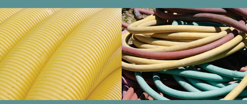
Environmental factors can damage hoses. Hoses on equipment stored indoors (away from sun, heat, rain, ice, and snow) should last longer than hoses on equipment stored outdoors. That's why some companies remove hoses from outdoor equipment and store them inside.
