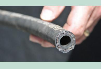
Second, hoses fail from the outside, in. How long a hose will last depends on its quality, what it is used for, and if it remains outdoors year round. For instance, a hose that remains straight will last longer than one that has been folded and unfolded, kinked and unkinked. A discharge hose continually dragged on gravel or pavement without a plastic cover will break down quicker than one protected by a plastic coil or covering.
