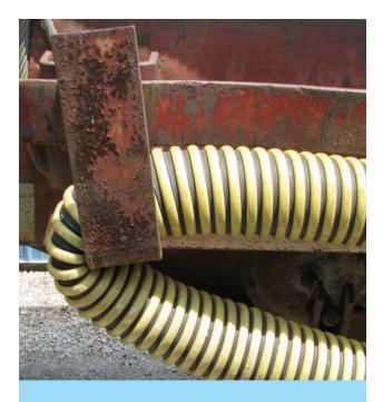
Make sure a hose does not go beyond its bending radius to keep it from failing prematurely or having its flow restricted. Hose splices are not recommended. The fitting used to fix this hose break (below) will restrict product flow.
