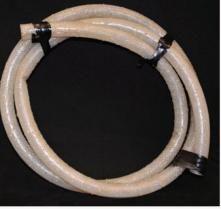
Certain chemicals can quickly degrade hoses (such as blistering) and cause them to fail. The herbicide in the tank shown here deteriorated the site gauge hose, leading to a spill that went into the city's sewer treatment plant.
