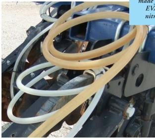
Consider rubber hoses: they may all appear to<br/>be similar, but there are many different blends of<br/>rubber hoses. EPDM (ethylene-propylene-diene-<br/>terpolymer) rubber hoses are inexpensive, durable,<br/>strong, and compatible for most fertilizer and<br/>diluted chemical solutions. But petroleum<br/>products cause EPDM hoses to fail. So if you<br/>plan to use a rubber hose to carry petroleum<br/>products, use one made of nitrile rubber.It's a<br/>storage<br/>hoses.
