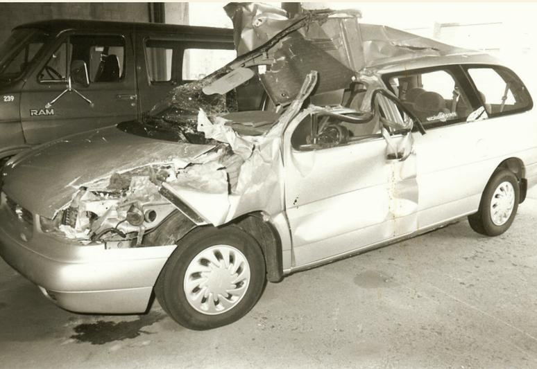
*The driver of this car had a harrowing experience with a trailer: “Here is my crash picture. The trailer, which was coming towards me, disengaged from the pickup. Then the hitch came straight up, into, and through the driver’s side (ripping the roof up), and launched into the air. After they cleared the scene, the fireman came over and told me, ‘Lady, you sure are lucky — you need to buy us lottery tickets today.’”*
