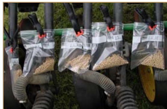
Figure 2. Seed captured during a calibration run over a known, fixed distance shown here prior to weighing.
