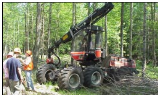
Modern logging equipment like this feller-buncher cuts the tree, bucks logs, and piles logs to be picked up by another machine and hauled to log landing.
