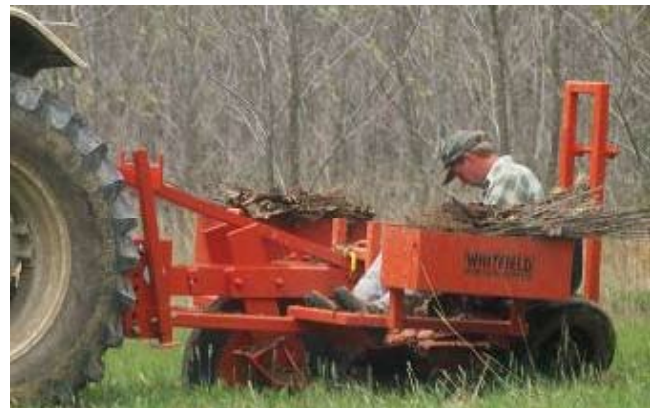
Figure 10. Tree planting machines increase tree planting production many fold over hand planting. Many forestry consultants use tree planting machines.
