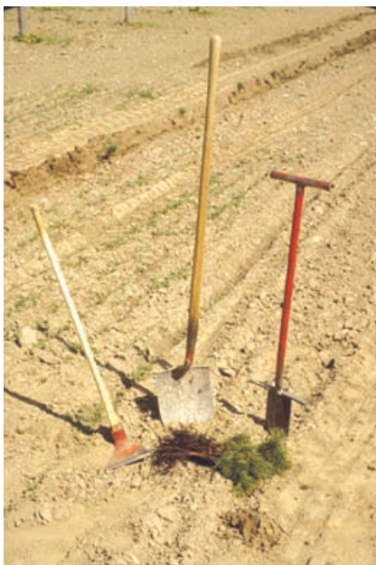
Figure 9. Hand tools commonly used for tree planting. Left to right are a mattock, a garden spade, and a KBC bar.
