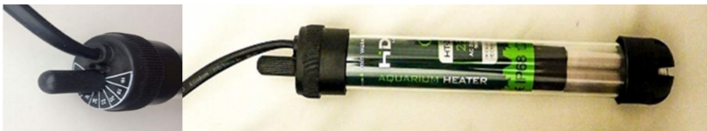
Figure 4. Aquarium heater used for increasing the temperature of nutrient solution inside the reservoir. Note the dial for temperature set points on the aquarium heater.
