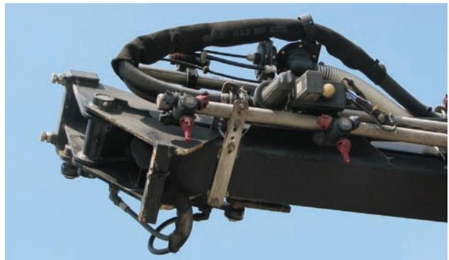
*Improperly installed hoses can kink and fail.*
