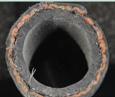
*Hoses can wear from the inside, out. Proper hose inspection includes hose interiors and exteriors. If the tube cover separates from the inner hose, it is time to replace the hose.*
