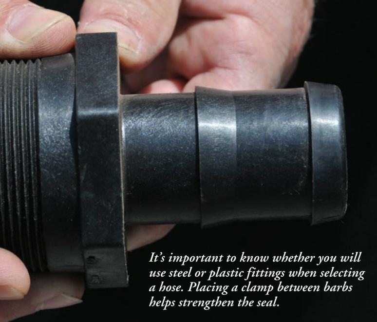
*It's important to know whether you will use steel or plastic fittings when selecting a hose. Placing a clamp between barbs helps strengthen the seal.*
