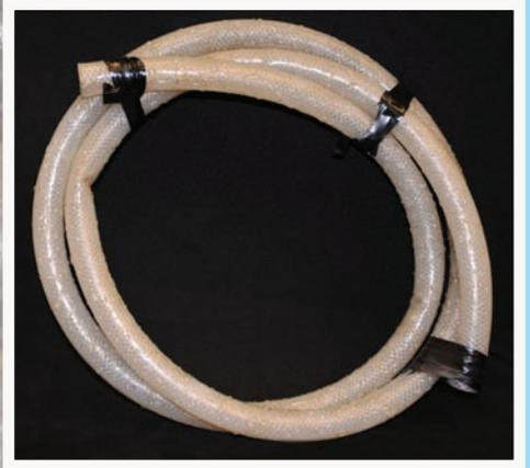
*Certain chemicals can quickly degrade hoses (such as blistering) and cause them to fail. The herbicide in the tank shown here deteriorated the site gauge hose, leading to a spill that went into the city's sewer treatment plant.*
