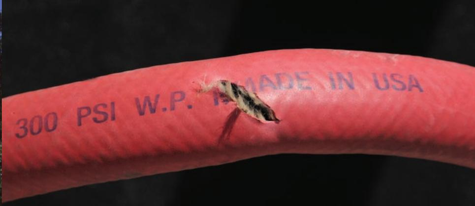
*The red hose shows sign of bursting under too much pressure. Some applications (left) require higher pressures than others (below). Never use a hose unless you are sure of its pressure rating.*
