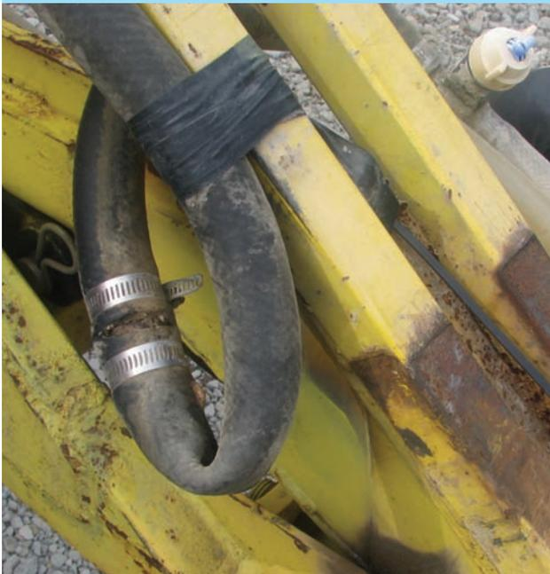
Bend radius measures how much a hose can bend without kinking and compromising its integrity. For instance, a hose with a 3-inch bend radius can bend around an object that is 6 inches in diameter (or more) without kinking.
