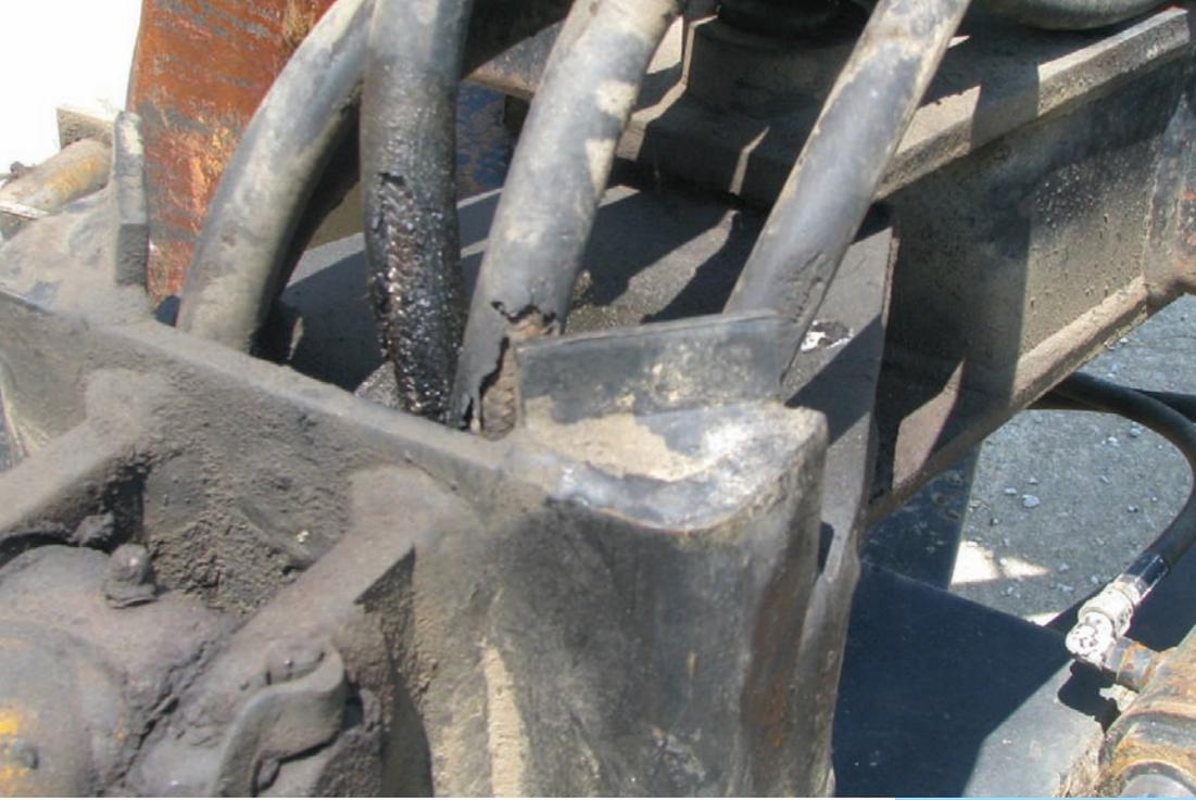
*Prevent petroleum products from getting on hoses — either by leaks or dripping. Petroleum products can degrade any hose cover.*
