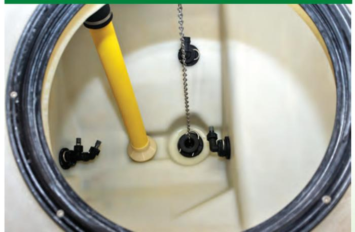
*Make sure to recirculate the hose reels at the beginning of the day. Materials may have settled in the bottom of the tank overnight.*
