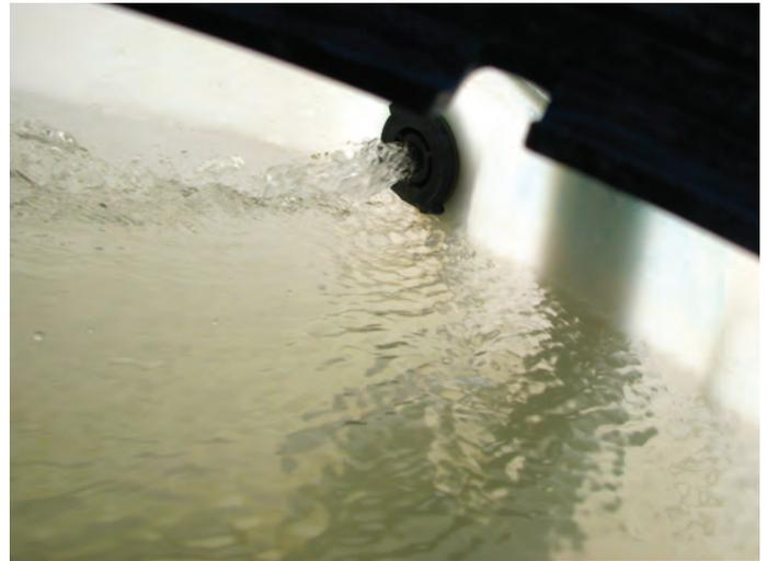
*Polyethylene (poly) tanks may employ pressurized bypass agitation to maintain a uniform mixture. In some cases, valves can be installed to better direct the incoming water at the bottom of the tank.*
