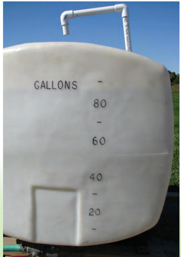
*Where is the 100-gallon mark on this 100-gallon tank? Tanks should be clearly marked for capacity.*
