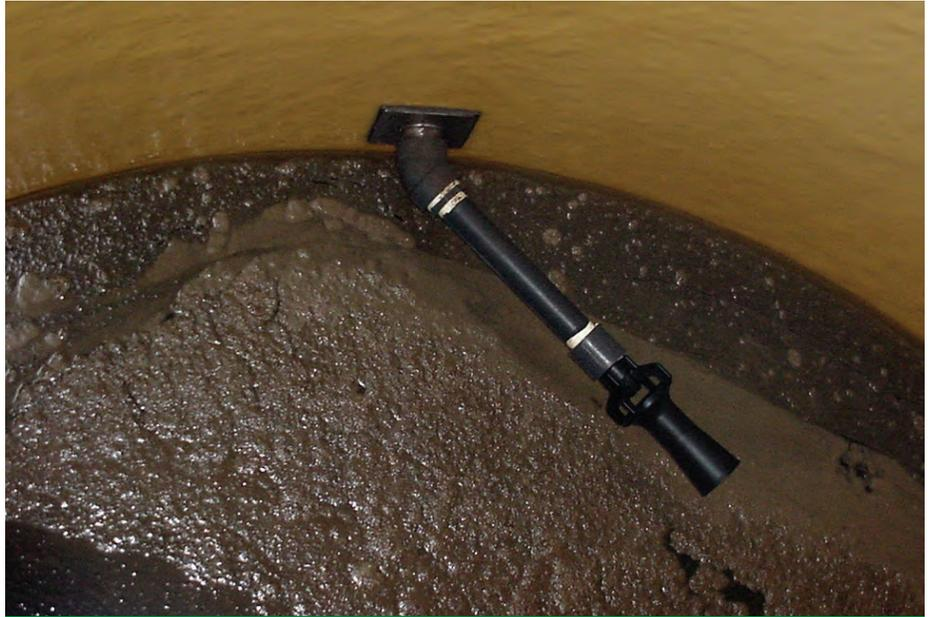
*Without agitation, product will settle at the bottom of the tank. As a result, solution taken from the bottom of the tank will have a much higher concentration of the product than solution taken from the top of the tank. This can lead to inconsistent results and unwanted damage.*
