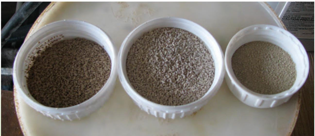
*The specific volume of a dry wettable granule (WG) pesticide product depends on its density. The volumes of WG products vary by their ingredients and the size and shape of their granules.*
