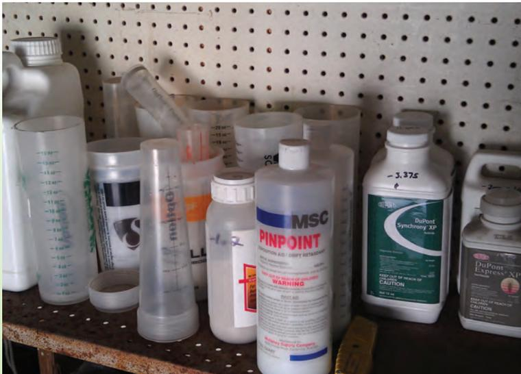
*Never use an old measuring tube for dry materials. Instead, properly dispose of or recycle all tubes after use. Saving them for reuse may lead to inaccurate measurements on future applications.*
