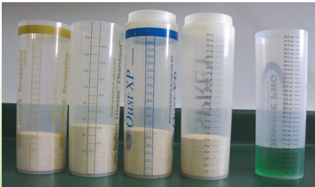
*These WG tubes clearly show how the graduations for measuring the weight of dry materials are product-specific. Each tube contains 6 dry ounces of product. For comparison, see 6 fluid ounces of the green liquid in the tube on the right.*
